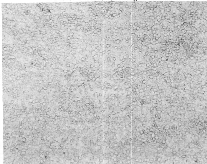
FIGURE 16. Ti-3Mn-COMPLEX ALLOY WITH 36 PPM OF HYDROGEN, SWAGED AT 1450 F AND STABILIZED
