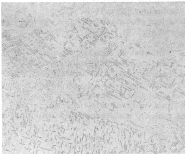
FIGURE 7. Ti-3Mn-COMPLEX ALLOY, ROLLED IN THE BETA-PHASE REGION, SOLUTION TREATED IN THE ALPHA-BETA-PHASE REGION, AND AGED
