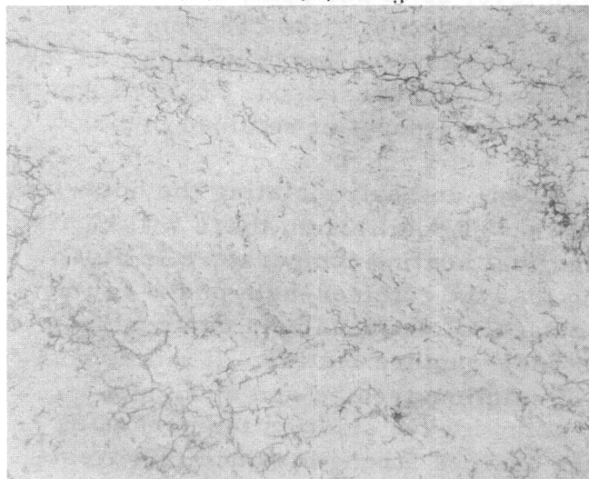
FIGURE 20. Ti-3Mn-COMPLEX ALLOY WITH 260 PPM OF HYDROGEN, ROLLED AND SOLUTION TREATED IN THE ALPHA-BETA-PHASE REGION AND AGED 48 HOURS AT 800 F; HEAVY ETCH ON COLD-DEFORMED GAGE SECTION OF SPECIMEN IN FIGURE 18
