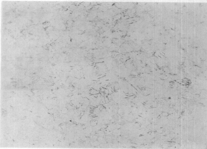
FIGURE 6 Neg. No. 34606 100X Electro polished Acetic glycol etch Alloy No. 75778 - Cold rolled to 0.059"
