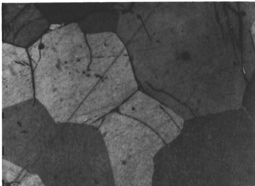
Figure 17. Hf-N: (77-23 At.%), Melting Point Sample Quenched from 2915°C. X800
