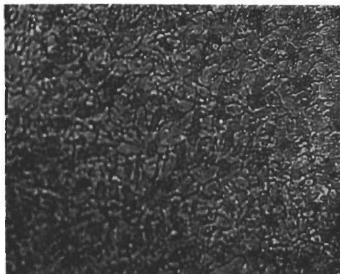
Figure 57. Hf-Ta-N: (20-40-40 At. %), Melting Point Sample Quenched from 2950°C. Polarized Light X 520 Primary Mononitride Dendrites (Light Gray) in a Subnitride-Mononitride Eutectic-Like Matrix.
