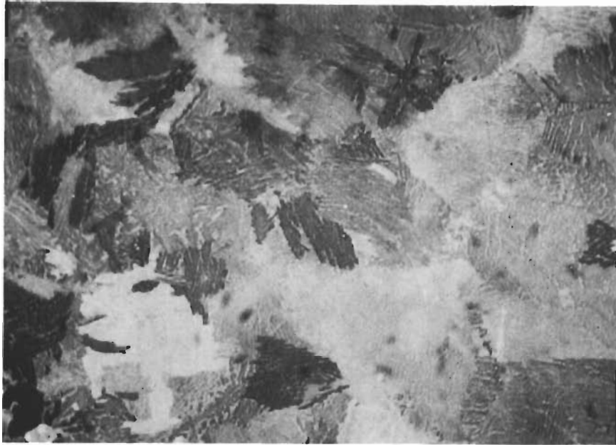
Figure 30. Hf-Ta-N: (75-23-2 At. %), Melting Point Sample Quenched from 2140°C. X440
