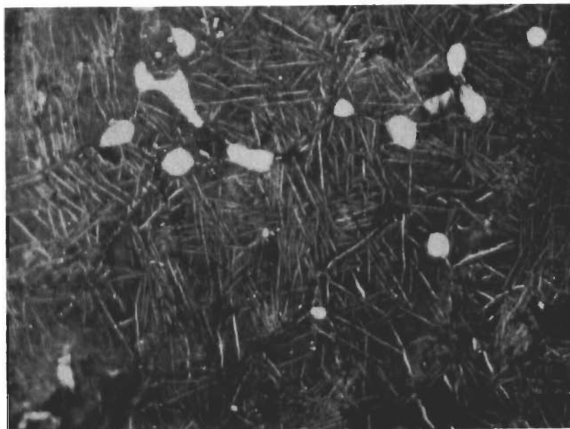
Figure 43. Hf-Ta-N: (20-75-5 At. %), Melting Point Sample Quenched from 2620°C. X1000
