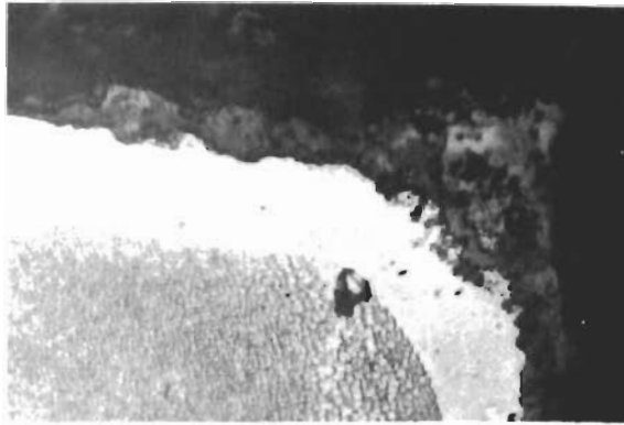
(a) Reacted for 52.5 hrs. in 1 atm. oxygen at 1000 °C. 500 x.
