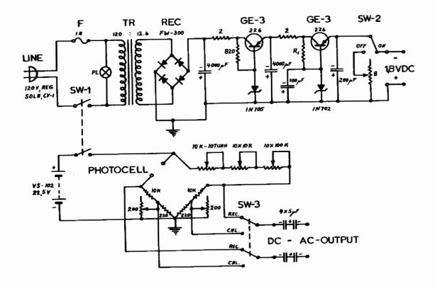
Figure 4. Regulated power supply for light bulb and photocell bridge circuit. The off-on switch, SW-2, connects with either the light bulb or a shunting resistance, 8, to permit turning the light on or off as a calibrating procedure. The switch, SW-3, in the bridge circuit drops the output signal to the recorder by a fixed fraction when turned to the calibrating (cal) position. This procedure is used in calibrating the opacity pulses in per cent of photoelectric current.
