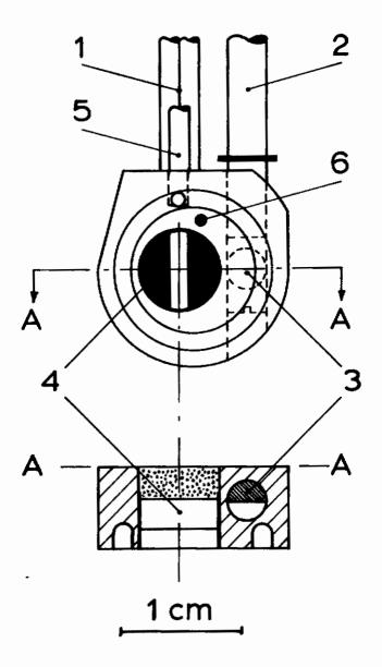
Prigure 2. Photoelectric plethysmograph for the oral mucosa, using fiber optics. Top section, seen from the mucosal surface: 1 - photocell lead, 2 - light wire, 3 - stainless steel mirror, 4 - photocell, 5 - tube connecting with groove to apply suction to the mucosa, 6 - thermocouple junction. Lower section, seen at 90° to the top section.
