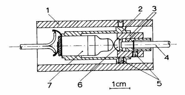
Figure 3. Light source, using pencil flash light bulb. 1 - plastic housing, 2 and 3 - brass housing, 4 - light wire, 5 - set screws, 6 - lens cut from light bulb, 7 - light bulb and mount.
