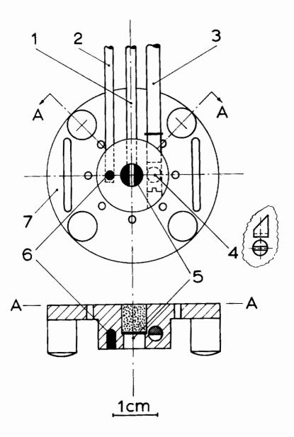
Figure 1. Cutaneous photoelectric plethysmograph with fiber optics.
