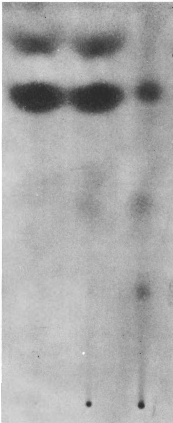
FIGURE 30 - THIN LAYER CHROMATOGRAM FOR 1-METHYL NAPHTHALENE BEFORE AND AFTER OXIDATION AT 400F
