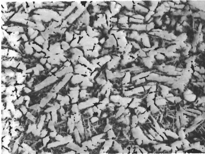
Figure 3. Zr-B (1.8 At% B), Quenched with \sim 80^{\circ}\text{C} per Second from 1790^{\circ}\text{C} .
