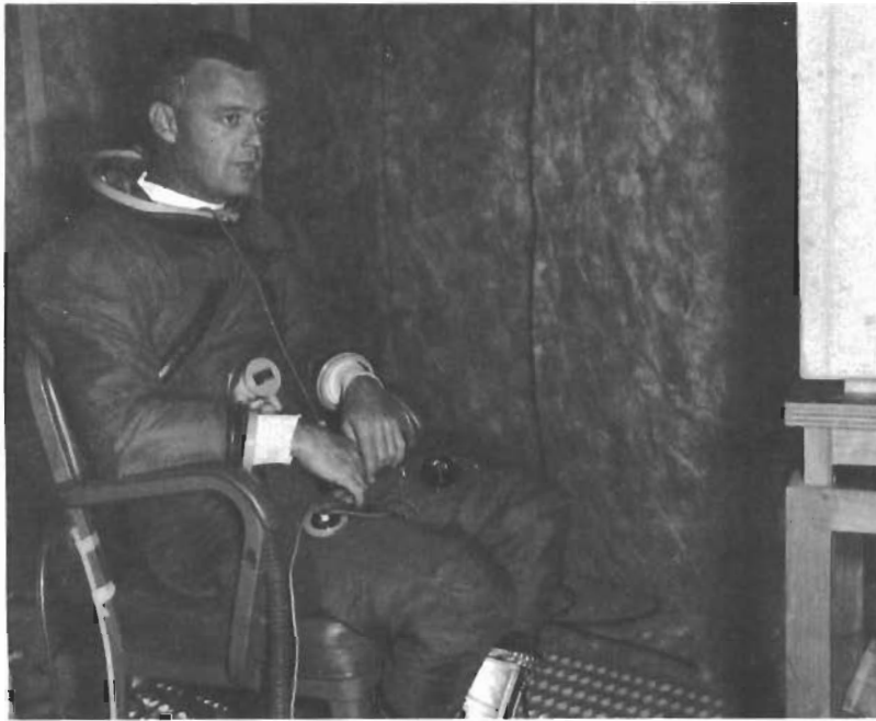
Figure 20. Measuring Noise Reduction at Ear
