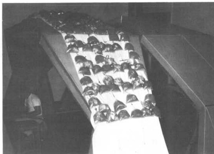
FIGURE 11. Concentrated load test - inverted "bow-tie" module.
