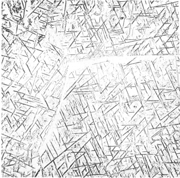
FIGURE 66. 4.64 PER CENT Cr ALLOY ISOTHERMALLY TRANSFORMED FOR 30 SECONDS AT 1202 F (650 C) Structure: Widmanstätten Alpha in a Beta Matrix
