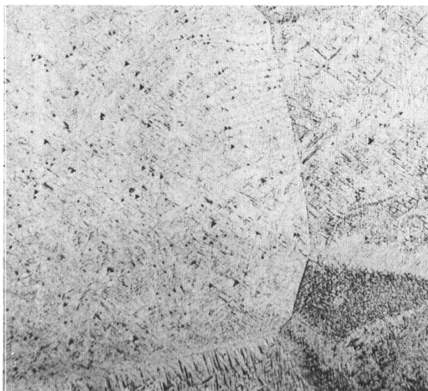
FIGURE 63. 4.64 PER CENT Cr ALLOY M_s DETERMINATION AT 842 F (450 C) Structure: Alpha-Prime Plates, Alpha and Beta
