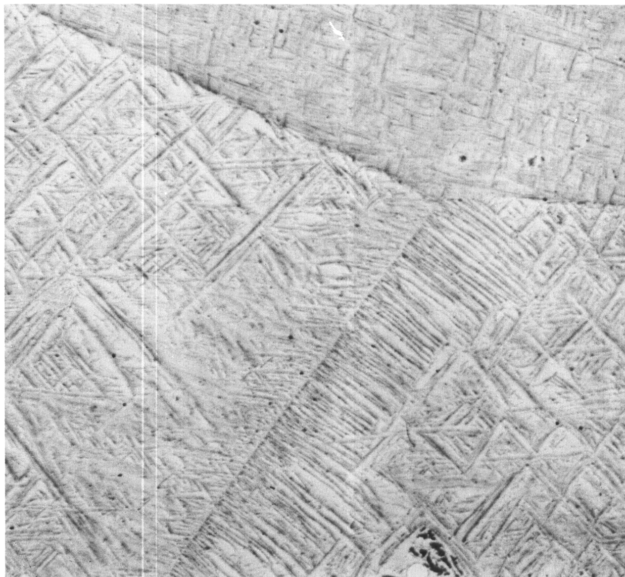
FIGURE 86. 7.54 PER CENT Cr ALLOY ISOTHERMALLY TRANSFORMED FOR 5 MINUTES AT 1022 F (550 C); A POSITIVE REPLICA, PLATINUM-SHADOWED ELECTRON MICROGRAPH
