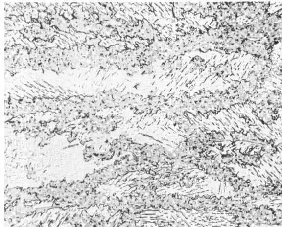
FIGURE 24. 10 PER CENT Cr ALLOY COLD ROLLED 31 PER CENT AND ANNEALED 60 HOURS AT 1112 F (600 C)
