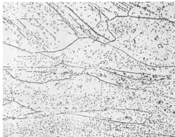
FIGURE 26. 20 PER CENT Cr ALLOY COLD ROLLED 30 PER CENT AND ANNEALED 1/4 HOUR AT 1292 F (700 C)
