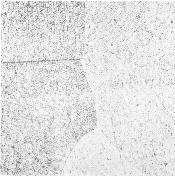
FIGURE 52. 7.54 PER CENT Cr ALLOY ISOTHERMALLY TRANSFORMED FOR 10 MINUTES AT 1022 F (550 C) Structure: Widmanstätten Alpha in a Beta Matrix
