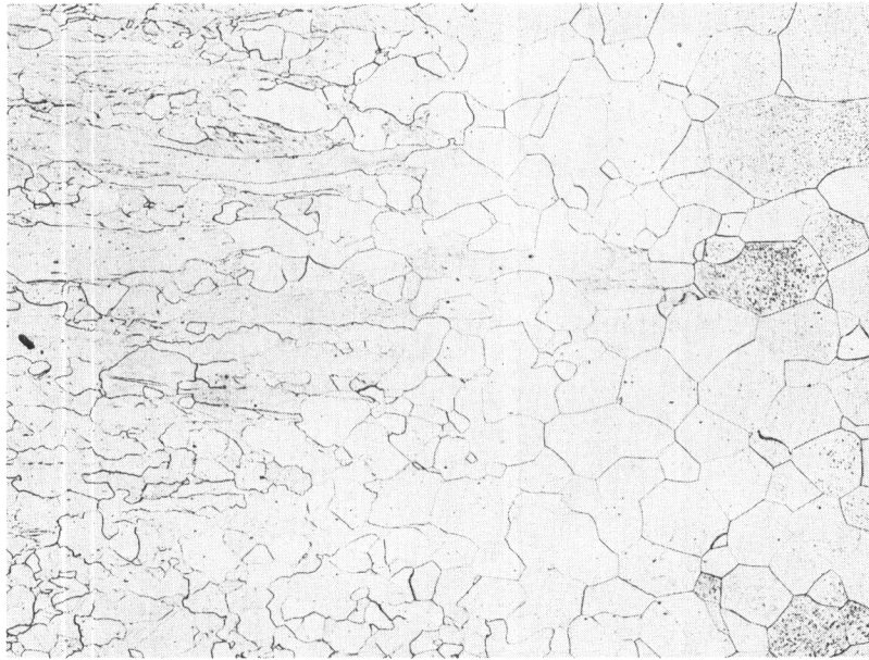
FIGURE 91. ARC-WELDED Ti-15 PER CENT Cr ALLOY, SHOWING SINGLE-PHASE BETA STRUCTURE OF BASE METAL (AT LEFT) AND BEGINNING OF HEAT-AFFECTED ZONE
