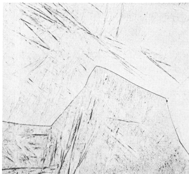
FIGURE 63. 4.64 PER CENT Cr ALLOY M_s DETERMINATION AT 842 F (450 C) Structure: Alpha-Prime Plates, Alpha and Beta
