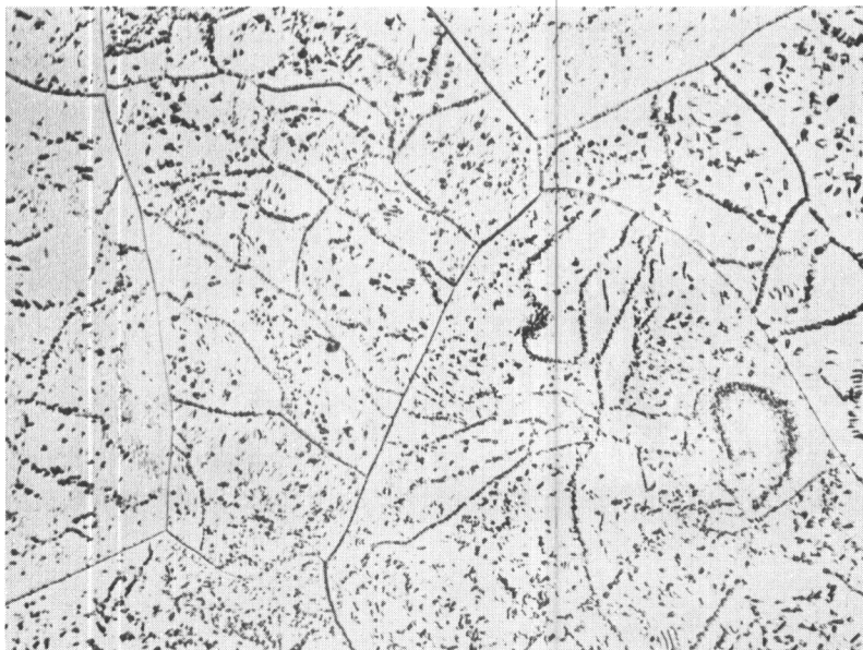
FIGURE 94. ARC-WELDED Ti-15 PER CENT Cr ALLOY SHOWING STRUCTURE OF WELD METAL AT HIGHER MAGNIFICATION
