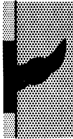
Development - Developer Acts Like A Blotter To Draw Penetrant Out Of Cracks
