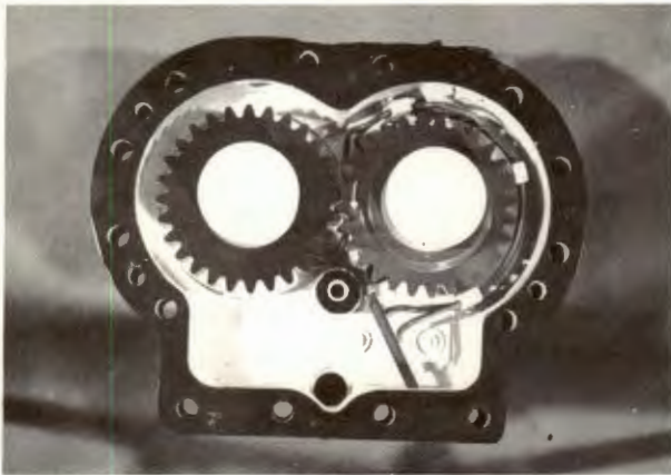
FIGURE 8. HOT GEAR RIG END COVER, INTERNAL VIEW
