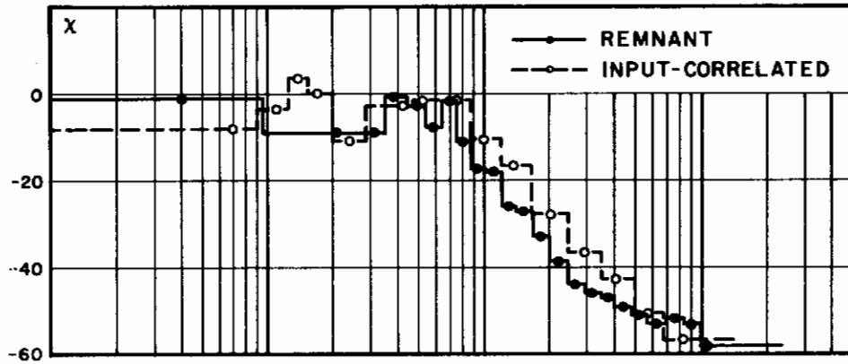
FIG. 14a POWER DENSITY SPECTRUM OF x(t) FOR \alpha = 8.0 SUBJ JM (0dB=1 FT 2 /RAD/SEC)
