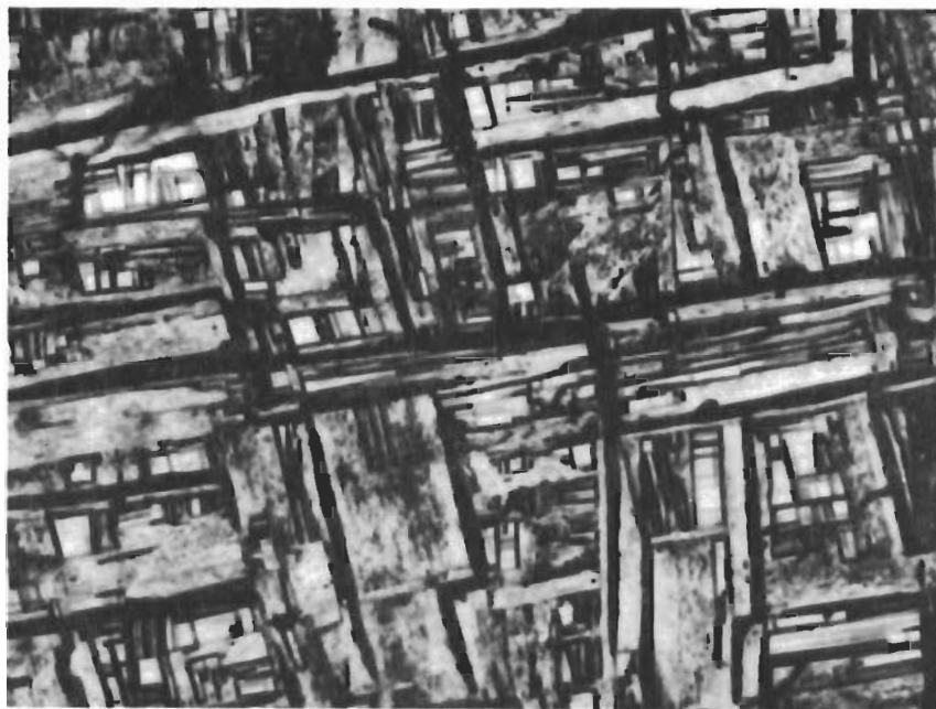
Figure 43. Mo-C (45 At% C), Sample from Figure 42, X1000 Equilibrated for 25 Hours at 1550°C and Quenched. \beta\text{-Mo}_2\text{C} with Graphite on Subgrain Boundaries
