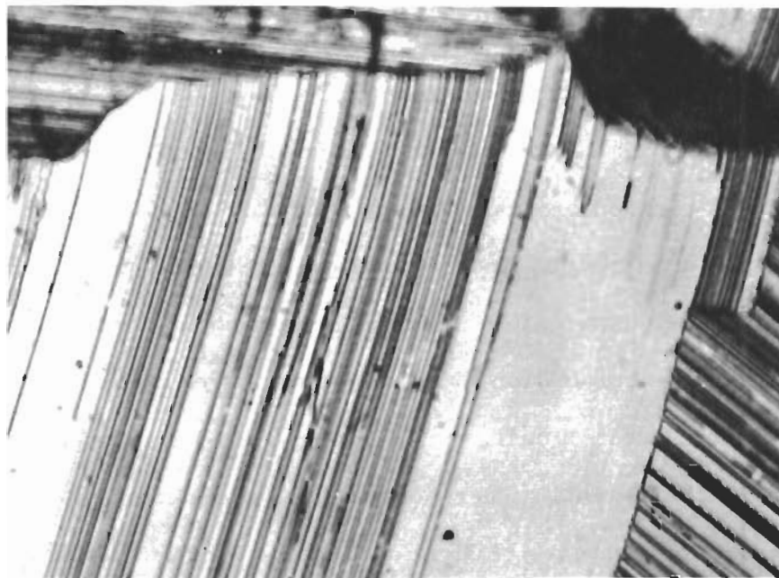
Figure 39. Mo-C (35.8 At% C), Rapidly Quenched from X2000 2470°C. Localized Precipitations of \eta - \text{MoC}_{1-x} in Originally Homogeneous Matrix of \beta - \text{Mo}_2\text{C} .
