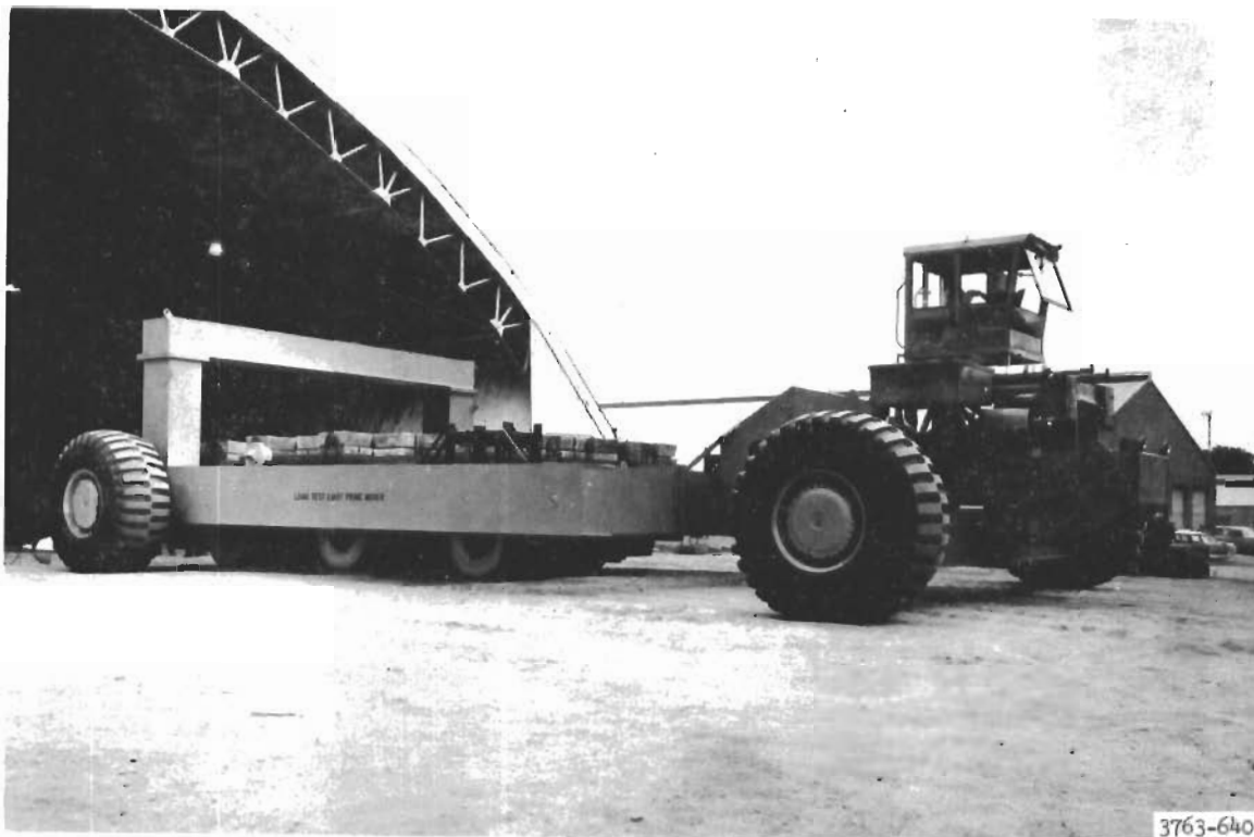
Figure 2. Test load vehicle used in trafficking lane 30
