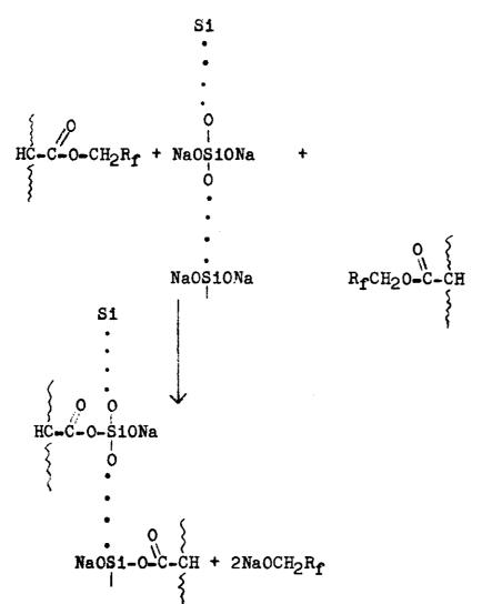
It is clearly evident that residual sodium silicate groups may be expected to contribute greatly to a decrease in the water resistance of the vulcanizate. Once again, no work has been performed on the theroetical aspect of the supposed mechanism.
