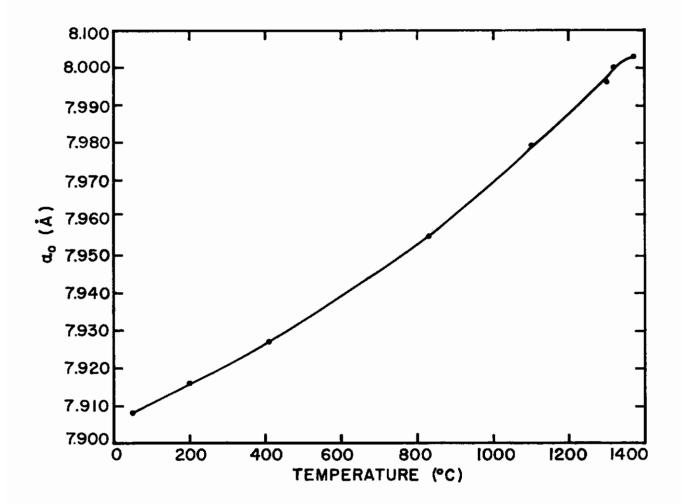
Fig. 1 Thermal Expansion of LiAl<sub>5</sub>0<sub>8</sub>
