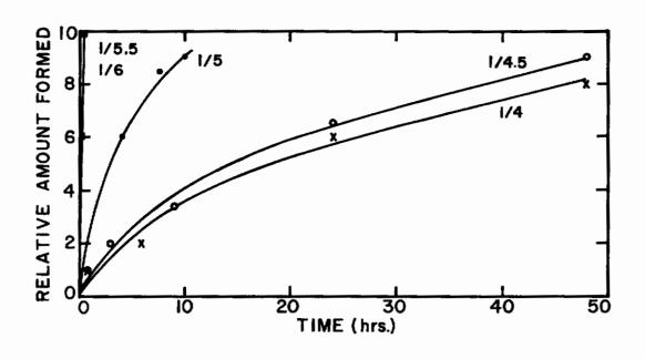
Fig. 3 Relative amounts of stable phase formed in lithium aluminates at  $900^{\circ}$  C. as a function of time (numbers on curves refer to  $\text{Li}_20$  /  $\text{Al}_20_3$  Molar ratios)
