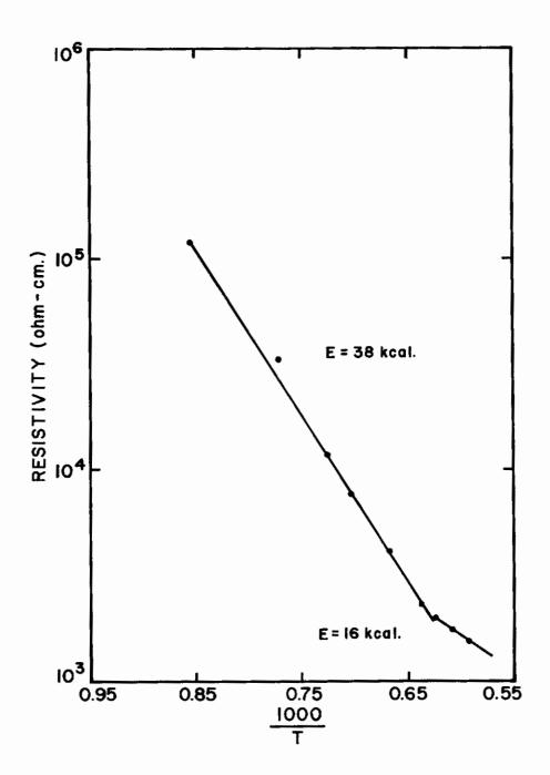
Fig. 2 Change in electrical resistivity of Li  ${\rm Al}_50_8$  with temperature
