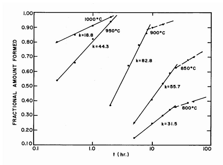
Fig. 5 Data from figure four replotted to fit diffusion equation -  $C = k \pmod{t}$
