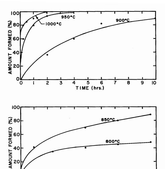
Fig. 4 Relative amount of stable phase formed in Li  ${\rm Al}_50_8$  as a function of time at different temperatures
