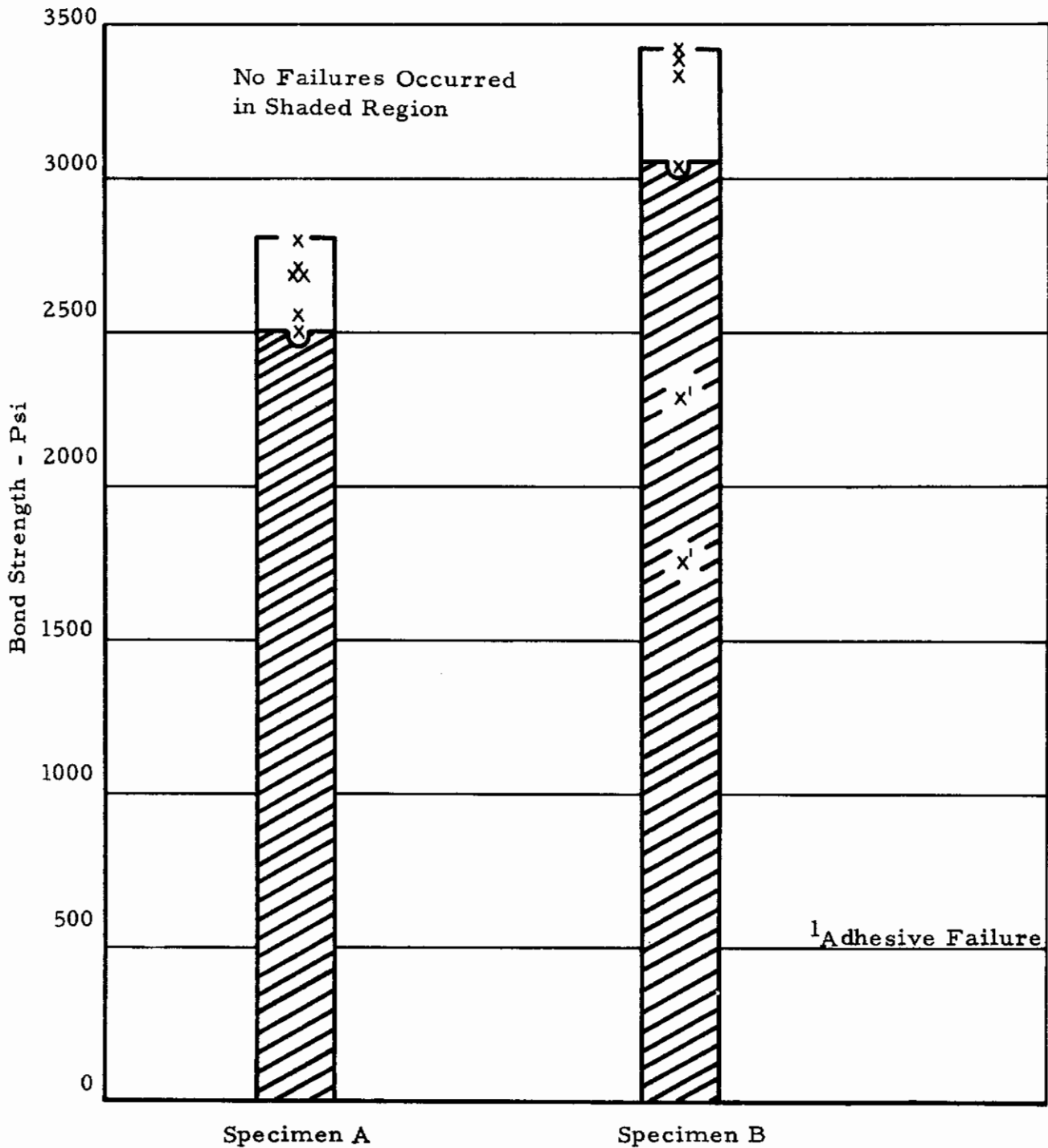
Figure 109. Bond Strength of Nichrome Graded ZrO_2 over Molybdenum Primed Stainless Steel for Two Methods of Sample Preparation.
