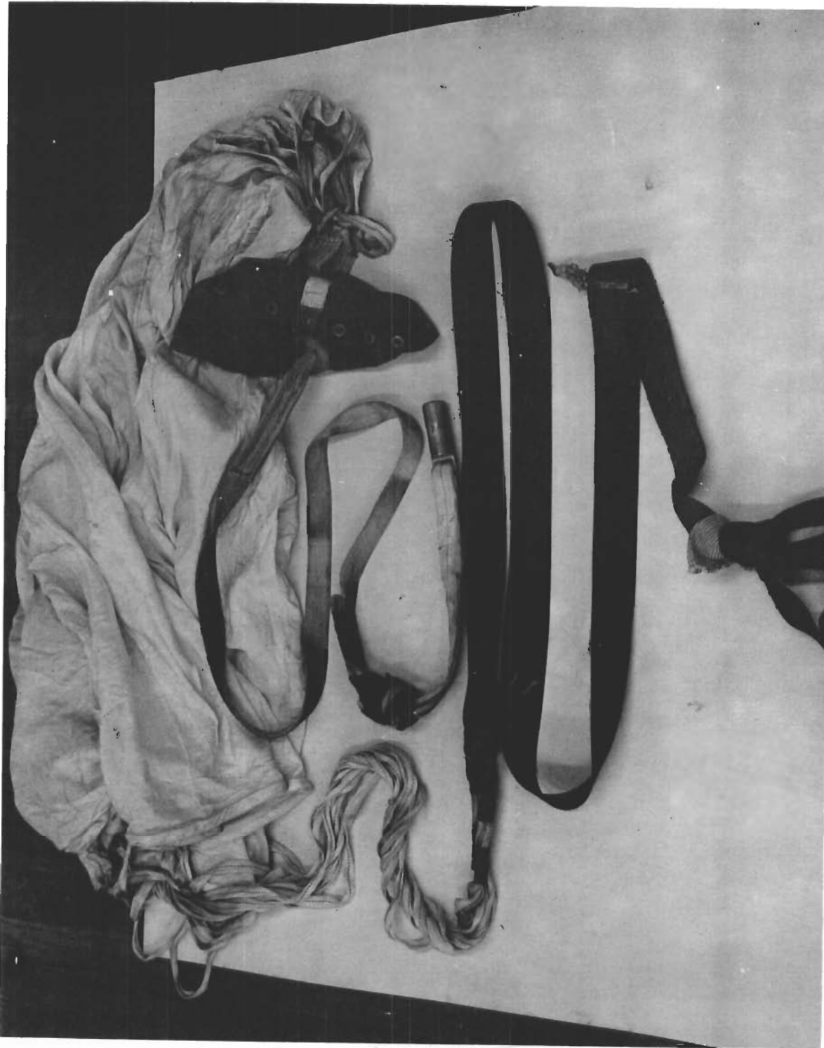
Figure 17. Recovery System Showing Drogue System and Attached Riser for Static Test
