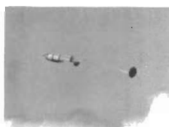
d. WITHDRAWAL OF RECOVERY - PARACHUTE BAG
