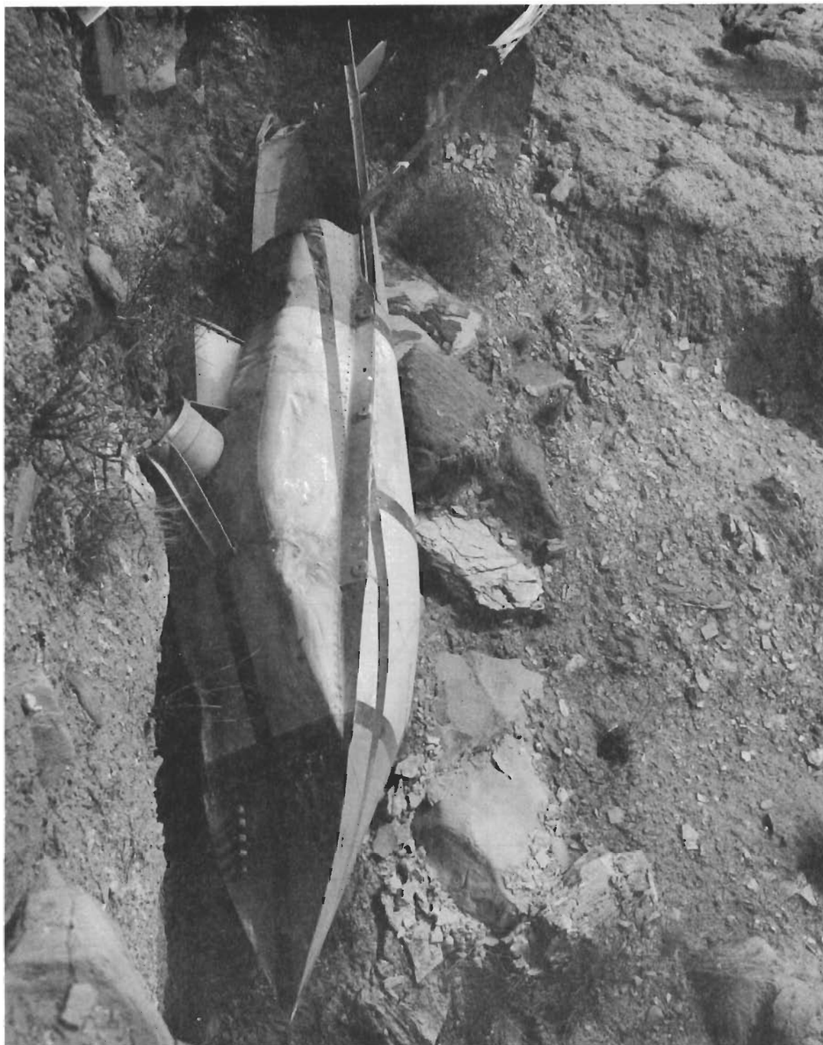
Figure 31. Side View of Capsule after Impact - Run Number 3
