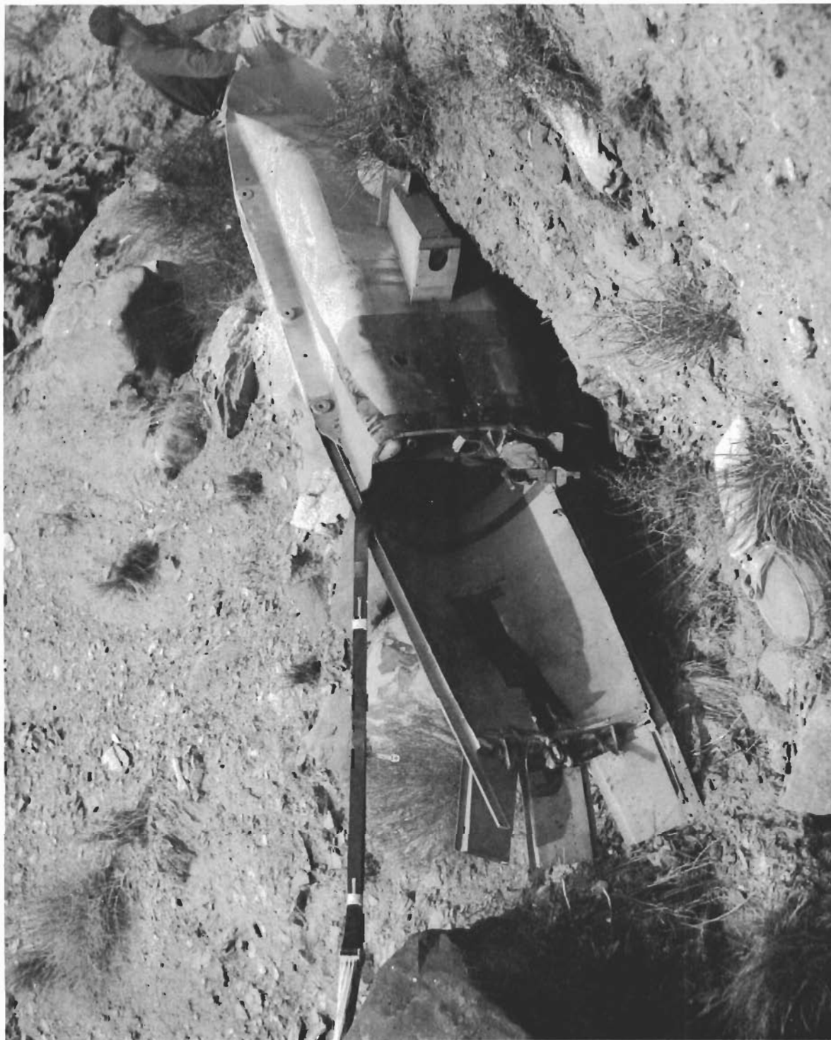
Figure 32. Three-Quarter Rear View of Capsule after Impact - Run Number 3
