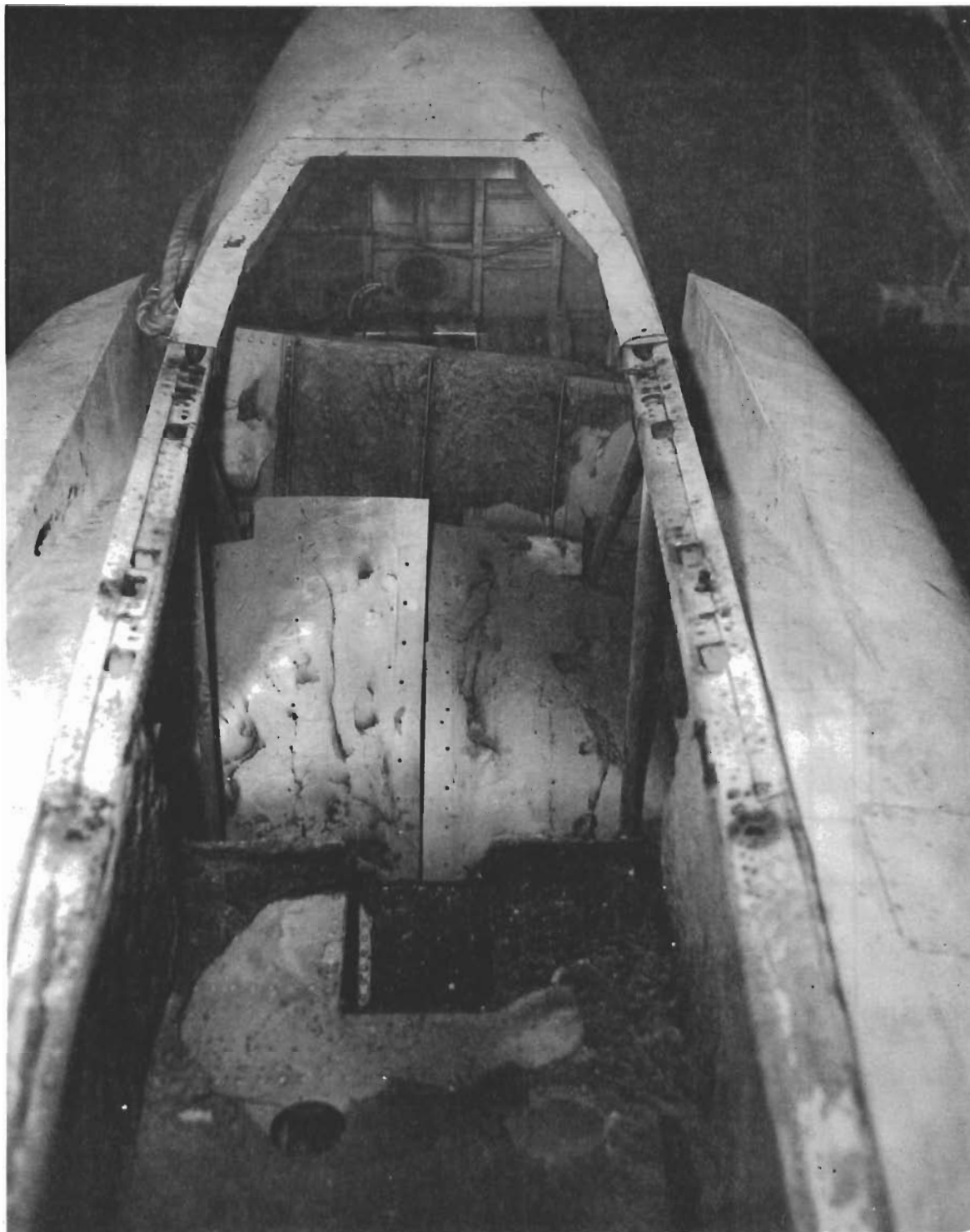
Figure 15. Rocket-Blast Effect on Interior of Vehicle - Static Test
