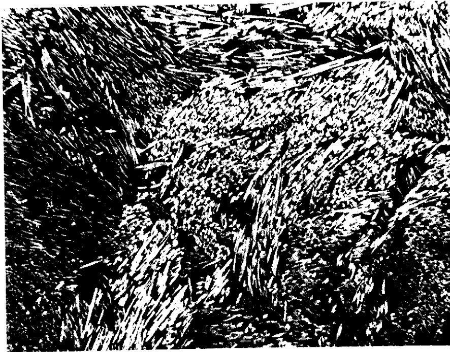
Figure 23. Photomicrograph of Macerated-Graphite-Cloth-Composites After Graphitization, With the Grain, (100X)
