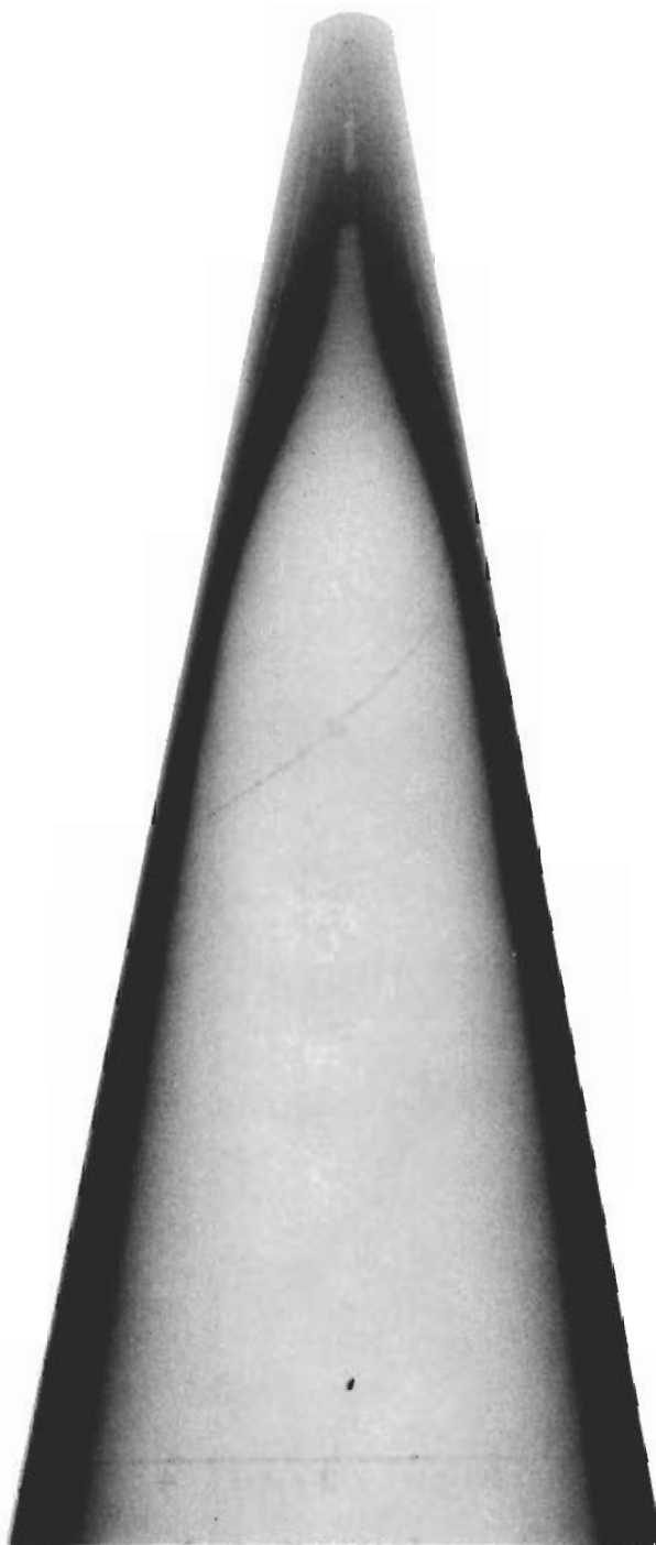
Radiographic Positive Nose Cone Tip 3213-4 (Nose Cone Tip 3213-3 with an additional 15 hours of deposition time).
