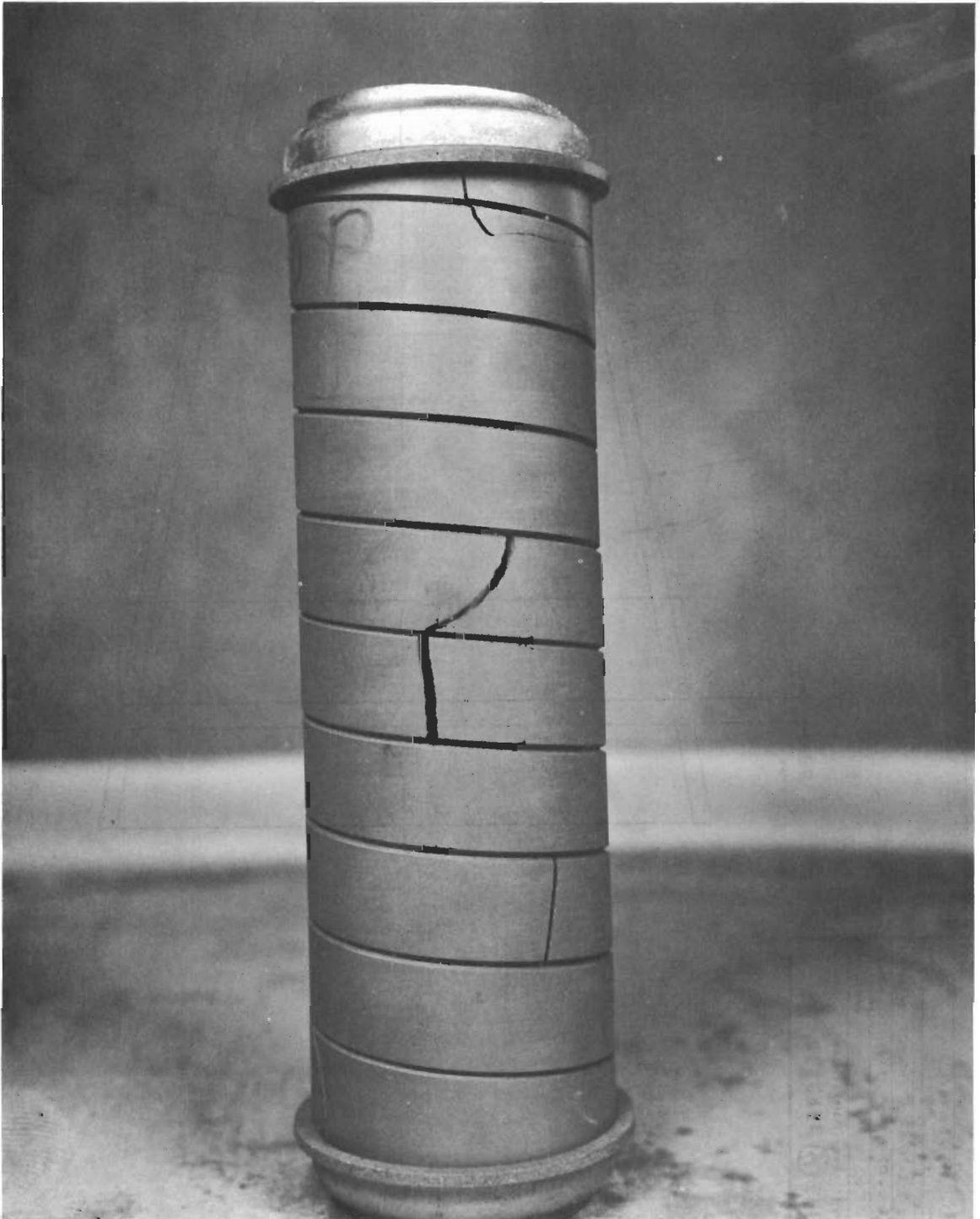
Typical Failure of Spirally Undercut Mandrel
