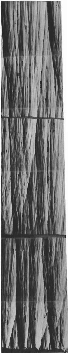
Photomicrographs Through the Deposit Thickness Showing Microstructure of Material from Top and Bottom of Frustum No. 2-108
