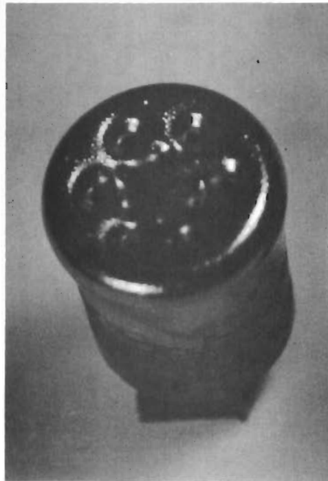
Nozzle Cap After Deposition
