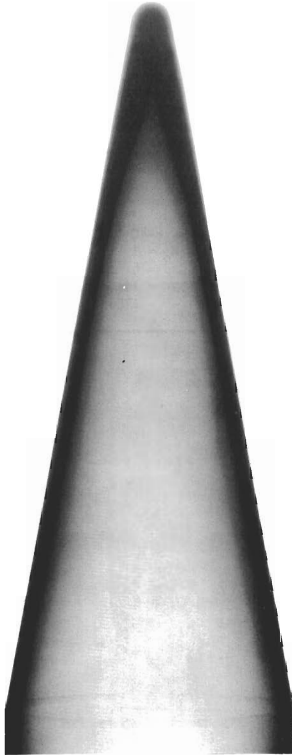
Radiographic Positive Nose Cone 1-43 Illustrating the General Growth Pattern
