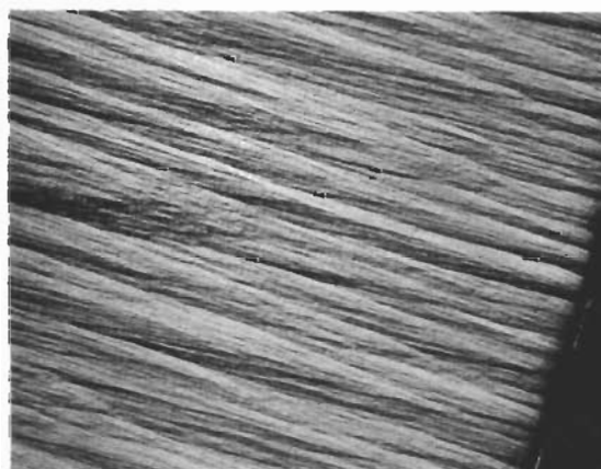
Microstructures of Tube Deposits Task 3.4.6 Orig. Mag: 50X
