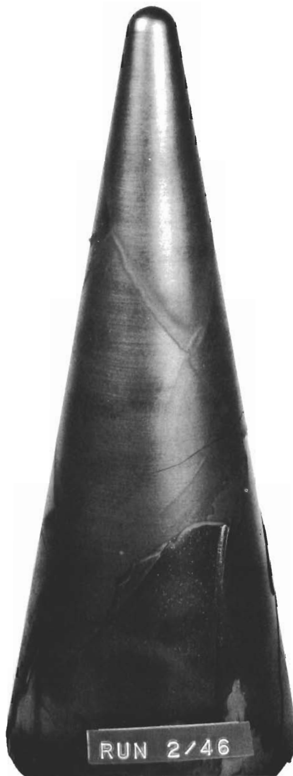
Photograph of Nose Cone 2-46 Illustrating Surface Condition and Overall Appearance Note Extremely Heavy Spallation Due to Residual Stresses Introduced by Process Fluctuations.
