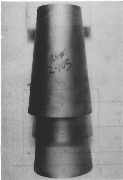
Illustrating excellent and complete separation between the three concentric frustum shells.
