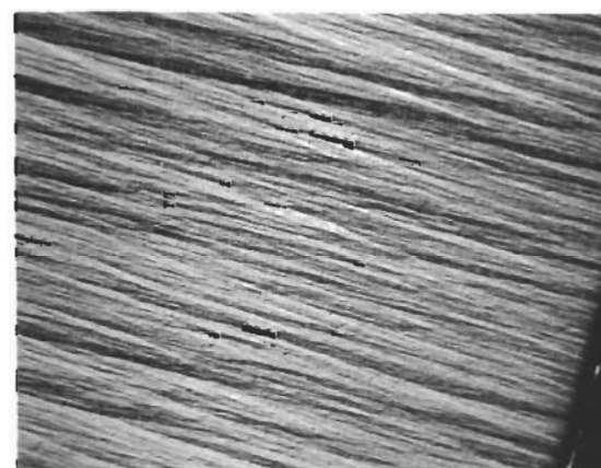
Microstructures of Tube Deposits Task 3.4.6 Orig. Mag: 50X
