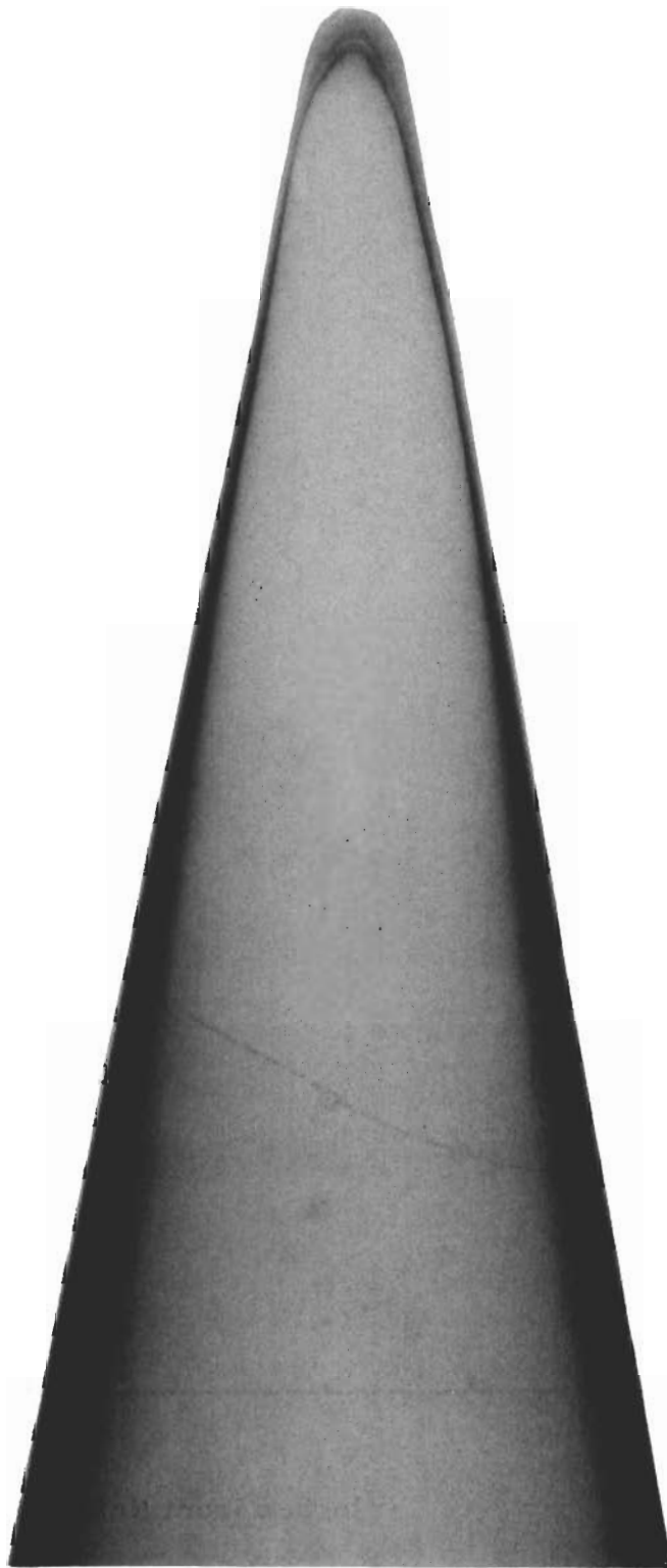
Radiographic Positive Nose Cone Tip 3213-2 Base Line Run No. 2 Nozzle Orifice 0.250"
