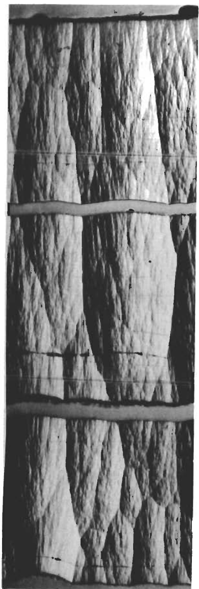
Photomicrographs through deposit thickness showing microstructure of material from the top and bottom of frustum 2-90
