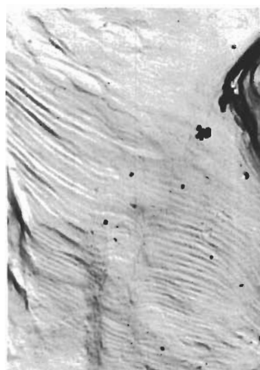
(A) FATIGUE AREA SHOWING STRIATIONS (19,000x)
