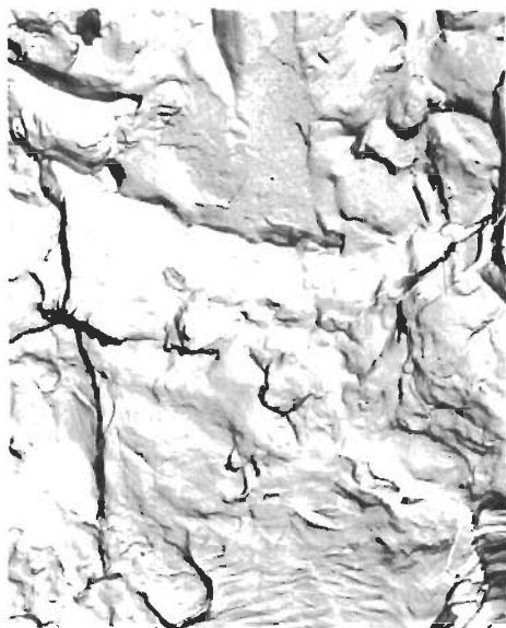
(C) TRANSITION ZONE FROM FATIGUE TO RAPID FRACTURE (1700x)
