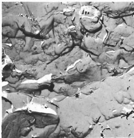
(A) PLANE STRAIN AREA OF RAPID FRACTURE (1700x)
