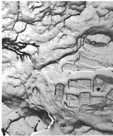
(A) INITIATION OF RAPID FRACTURE (1700x)
