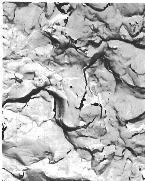
(A) TYPICAL AREA FROM PLANE STRAIN ZONE (1700x)
