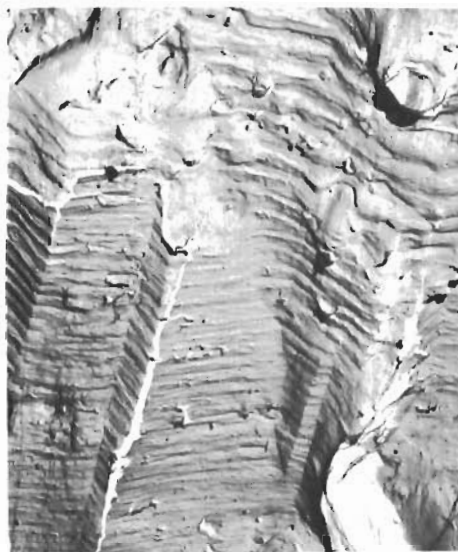
(C) STRIATIONS TYPICAL OF TWINNED MICROSTRUCTURE (1700x)
