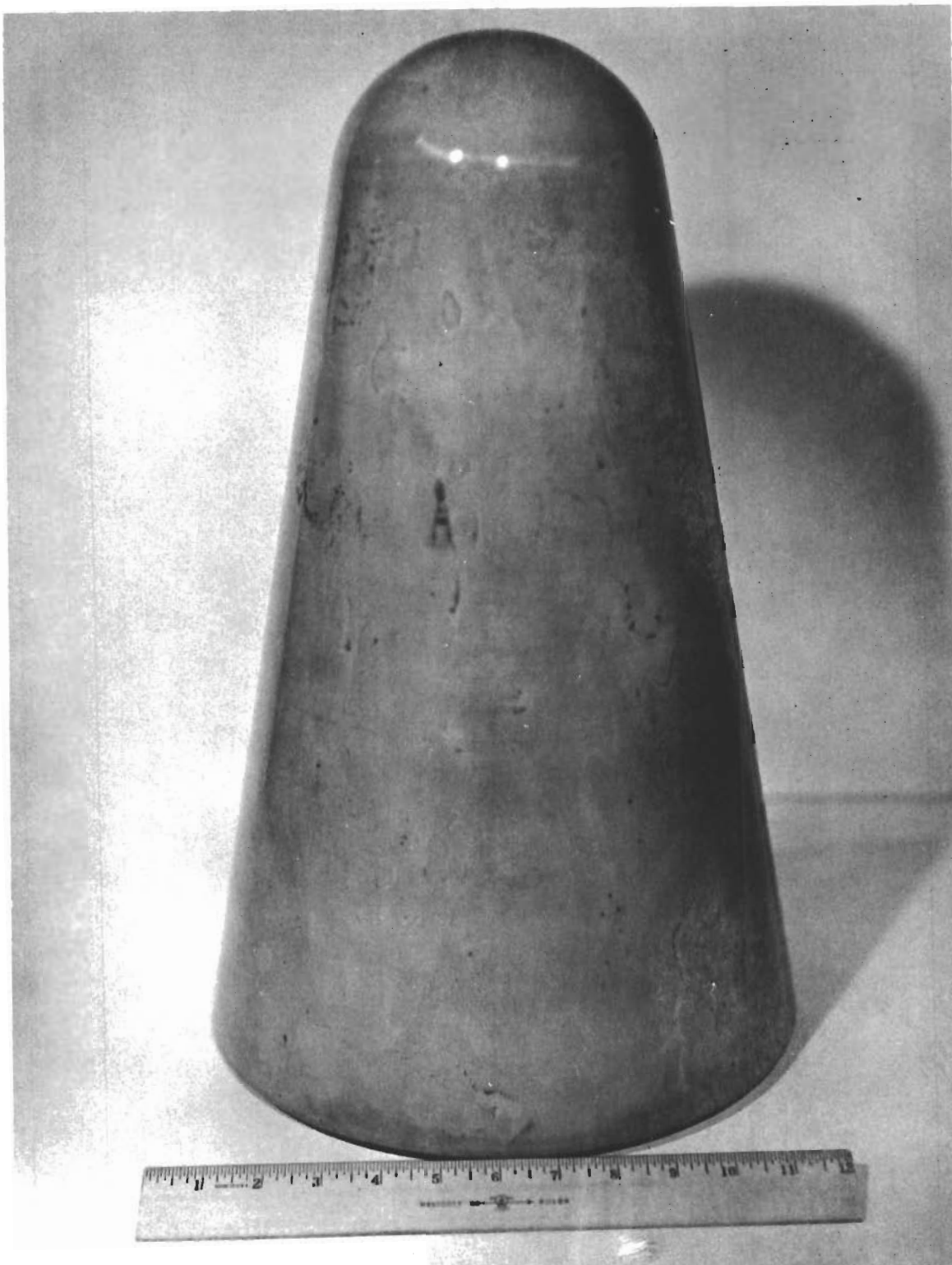
FIGURE 25. Plaster Mandrel for 500 square inch Nose Cone
