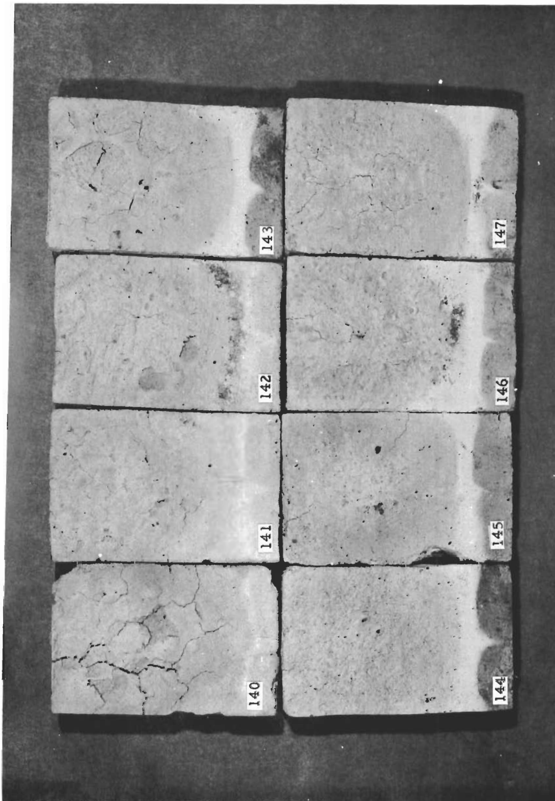
FIGURE 5. TherMarq ZSF-140 through -147 after 4000°F Exposure
