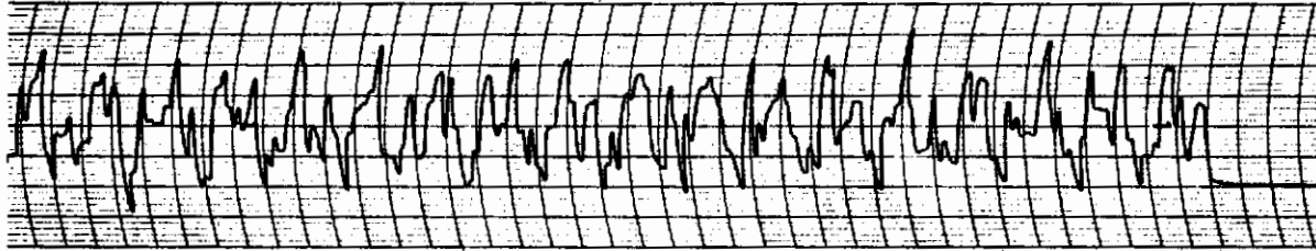
(a) "Easy" Forcing Function: - Filter Break Frequency = 1.50 rad/sec Paper Speed = 2 mm/sec
