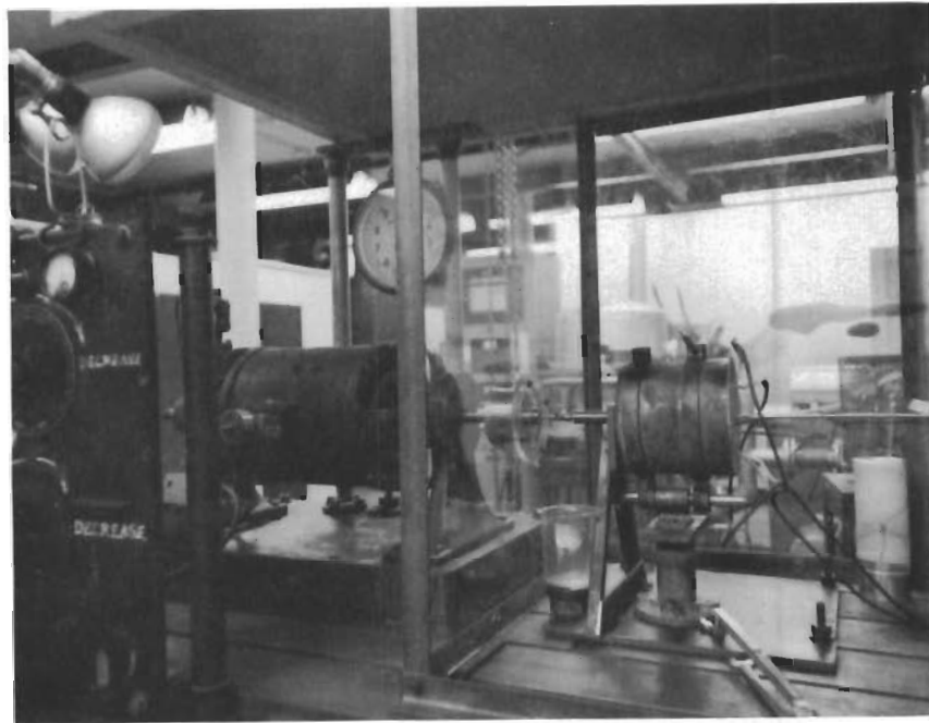
Fig. 21 COMPLETE APPARATUS FOR TESTING ROTATING SHAFT SEALS
