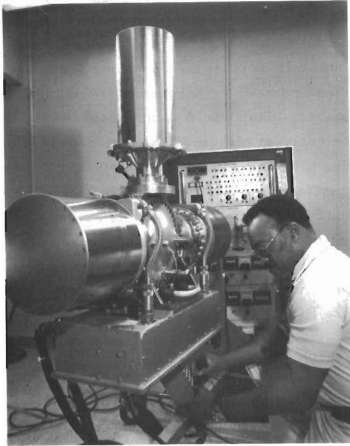
Figure 18. Hi Cap spaceborne VM refrigeration system (4S14027)
