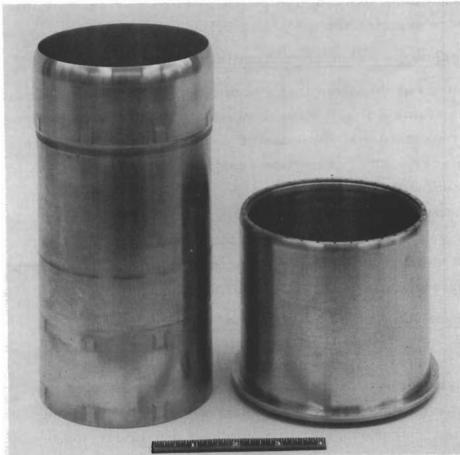
Figure 16. Cylinder ready to be plated (73-19400)
