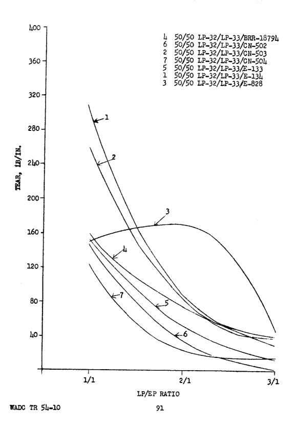
PROPERTIES OF EXPERIMENTAL "THIOKOL" LIQUID POLYMER/EPOXY RESIN INTEGRAL FUEL CELL SEALANT COMPOUNDS
