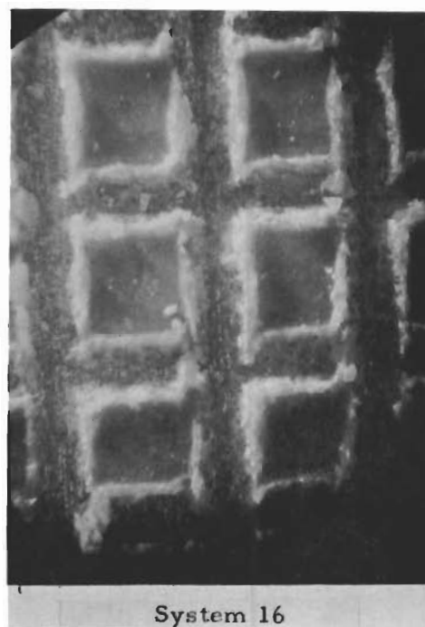
Fig. 24 ILLUSTRATIONS OF ADHESION PERFORMANCE OF COATING SYSTEMS 13 THROUGH 16
