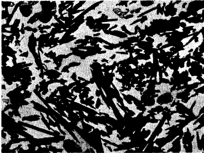
Figure 149. Sample from Figure 148, Re-equilibrated for 15 Minutes in the Liquidus + Solidus Region (2000°C), and Cooled. X900
