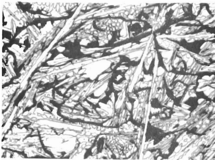
Figure 74 (b). Ti-B-C (33-21-46 At.%), Quenched from 2517°C. X1000
