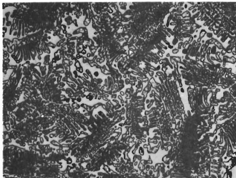
Figure 161. Hf-B-C (40-45-15 At.%), Quenched from 3145°C . X1000
