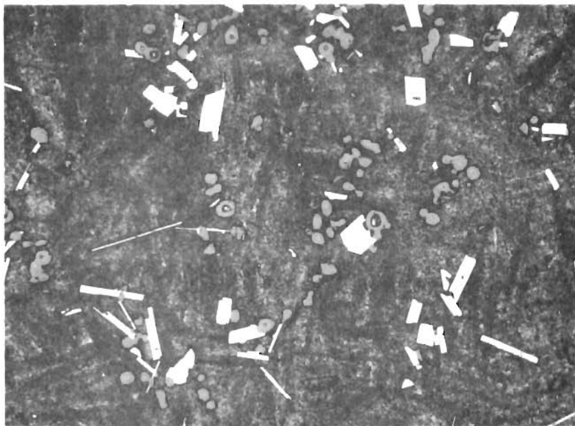
Figure 82. Zr-B-C (94-3-3 At.%), Cooled with Approximately 20°C per Second from 1700°C.
