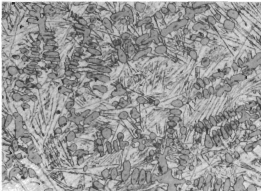
Figure 93. Zr-B-C (70-10-20 At.%), Quenched from 1800°C. X400 Increased Amounts of Primary Monocarbide, and Ternary Eutectic.
