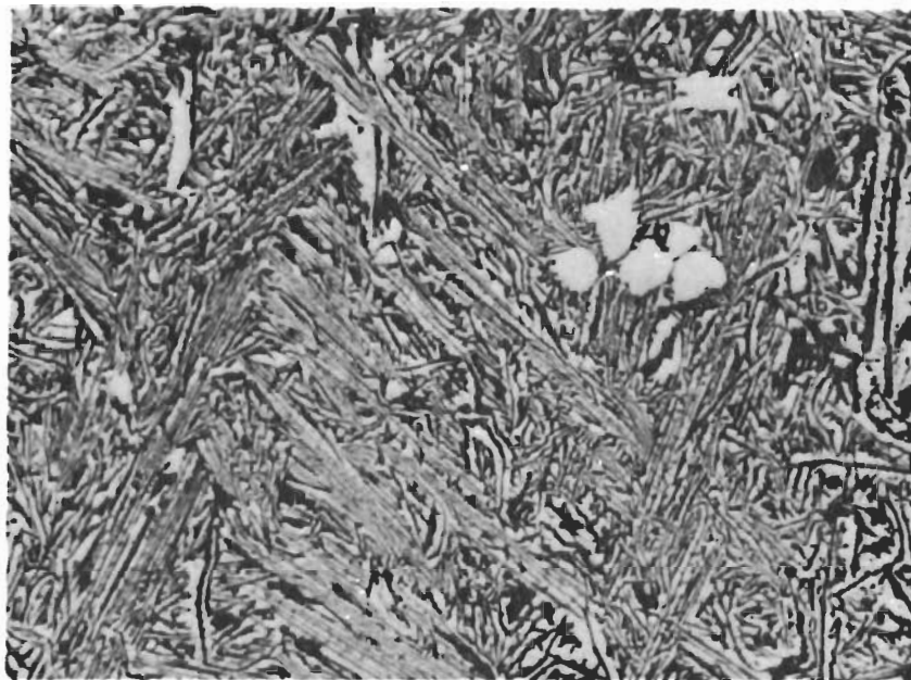
Figure 61. Ti-B-C (23-47-30 At.%), Quenched from 2514°C. X340 Traces of Primary Diboride in a Matrix of TiB_2 + C Eutectic.
