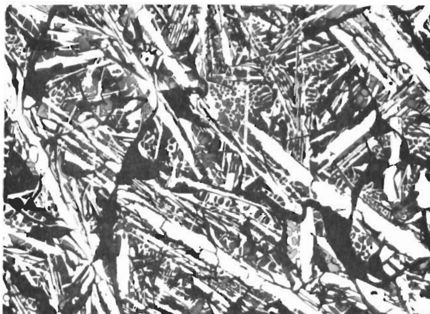
Figure 76. Ti-B-C (25-40-35), Cooled at Approximately 10°C per Second from 2430°C. X200
