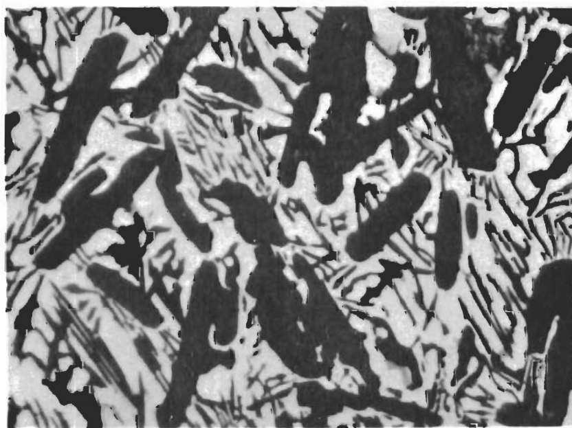
Figure 64. Ti-B-C (15-30-55 At.%), Cooled with Approximately 20°C per Second from 2640°C. X1000 Primary Graphite (Dark) in a Matrix of TiB 2 + C Eutectic.
