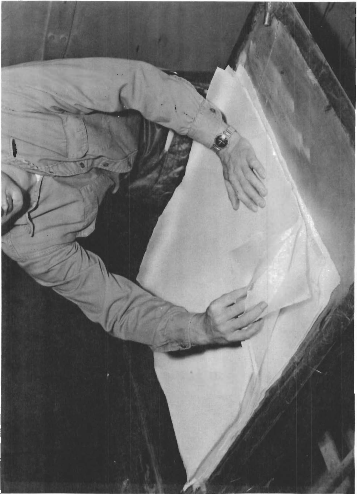
Figure 89. Glass Fiber Panel - Upper Surface Dry Fabric Lay-up
