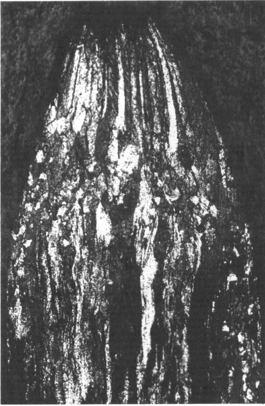
Fig. 131 2500 F Weld-zone Failure; X50; 0.050-in. Tungsten Weld
