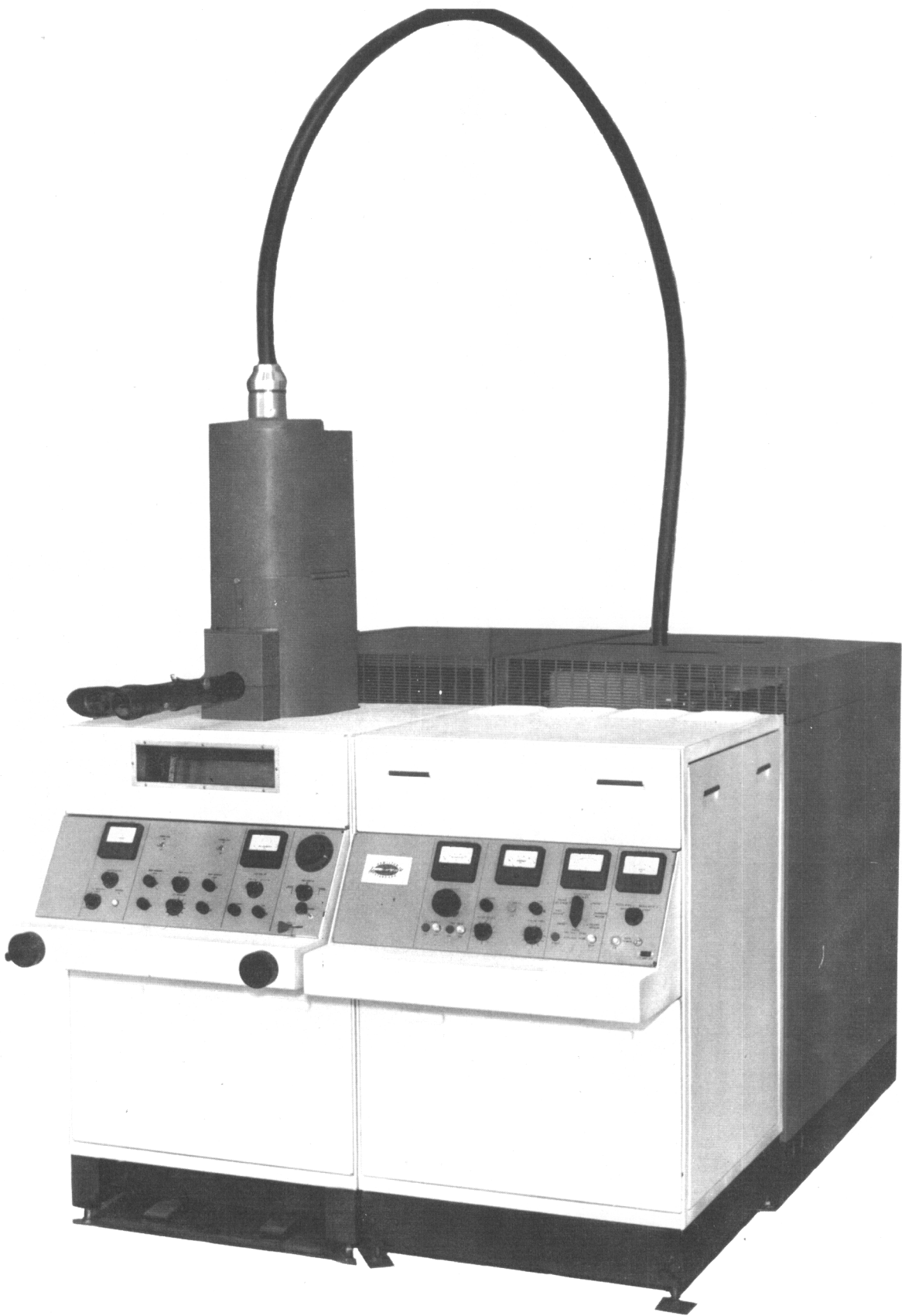
Fig. 13 Hamilton-Zeiss Electron Beam Welding Machine
