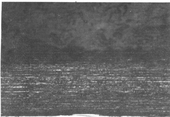
Fig. 27 As-received 0.100-in. Mo-0.5% Ti; X200
