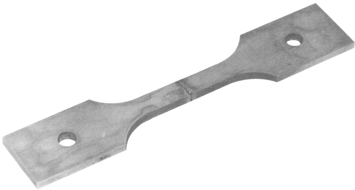
Fig. 2 Molybdenum Tensile Specimen
