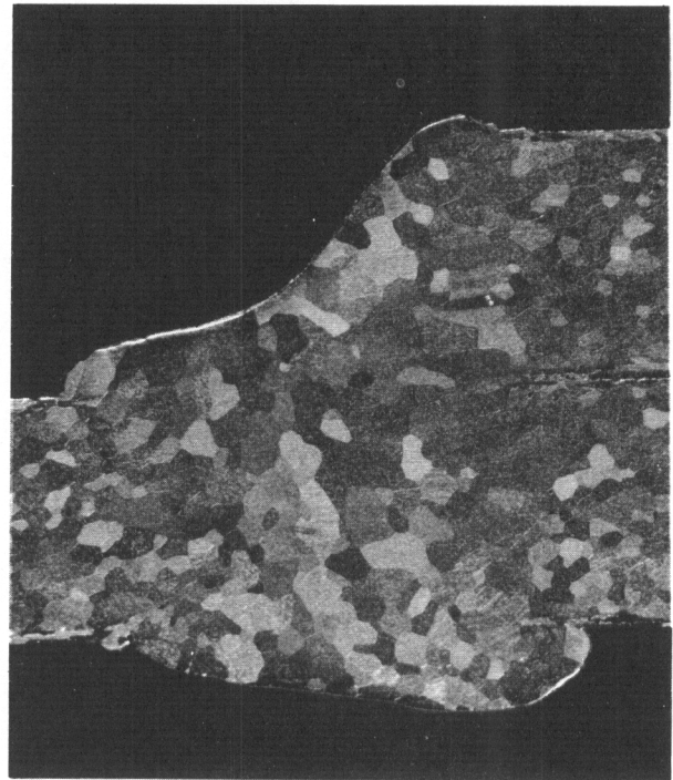
Fig. 114 Lap-weld Cross-section; X20; 0.055-in. Mo-0.5% Ti
