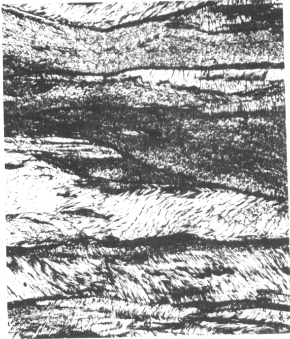
Fig. 31 As-received 0.050-in. Tungsten; X200
