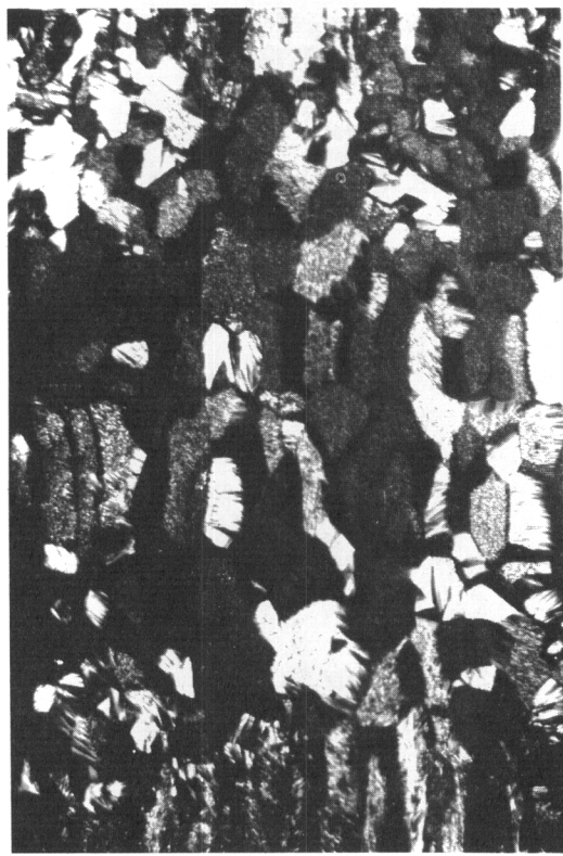
Fig. 104 Final Weld Microstructure; X100; 0.050-in. Tungsten
