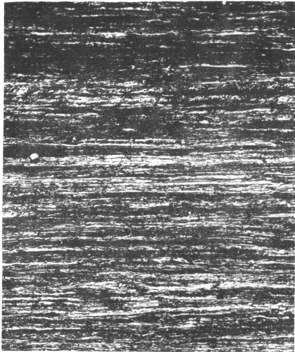
Fig. 27 As-received 0.100-in. Mo-0.5% Ti; X200
