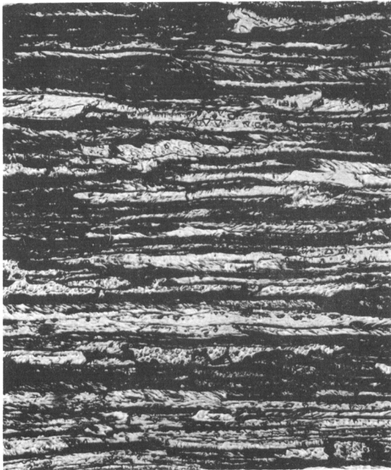
Fig. 25 As-received 0.055-in. Mo-0.5% Ti; X200
