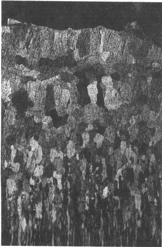
Fig. 126 Room-temperature weld-zone Failure; X50; 0.055-in. Mo-0.5% Ti Weld
