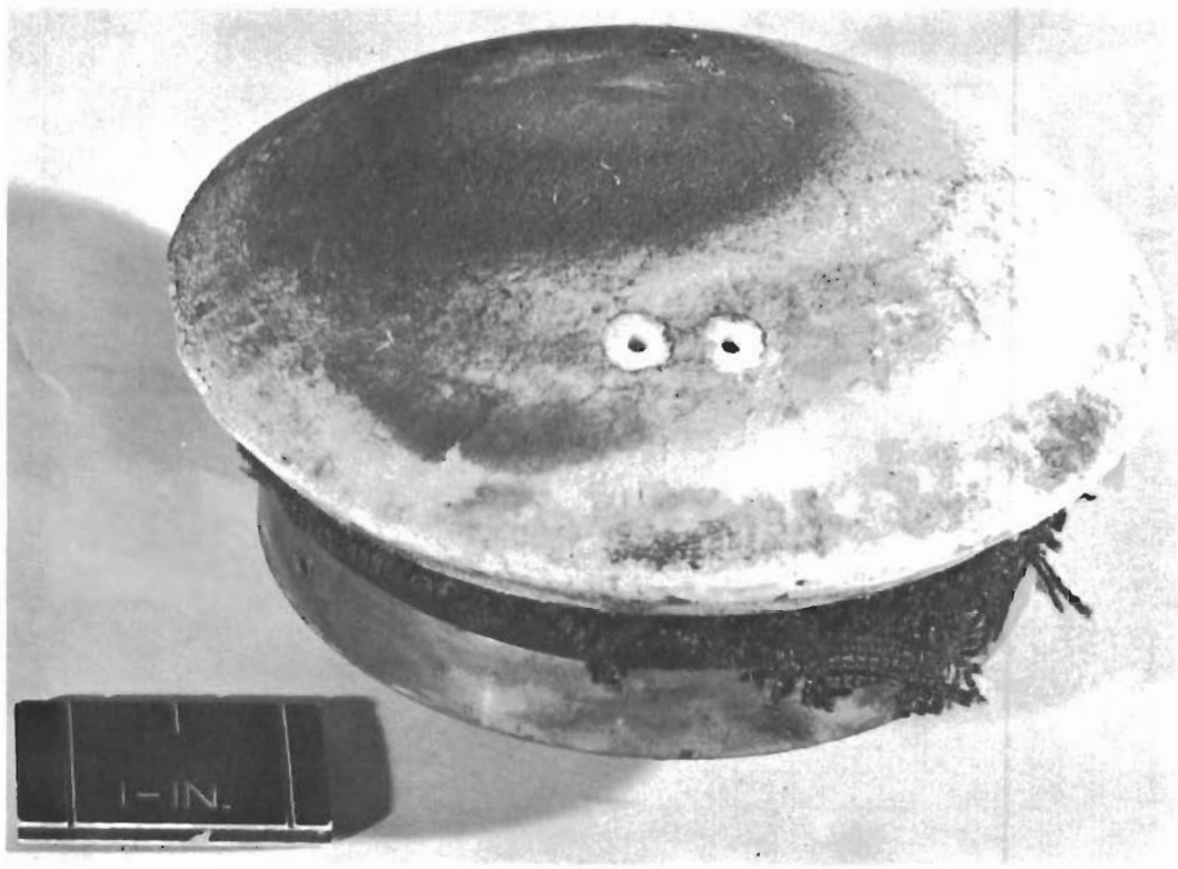
FIGURE 40. SO-71 + SO-84 COATED SUBSCALE ASSET SHAPE; After Plasma-Arc Testing
