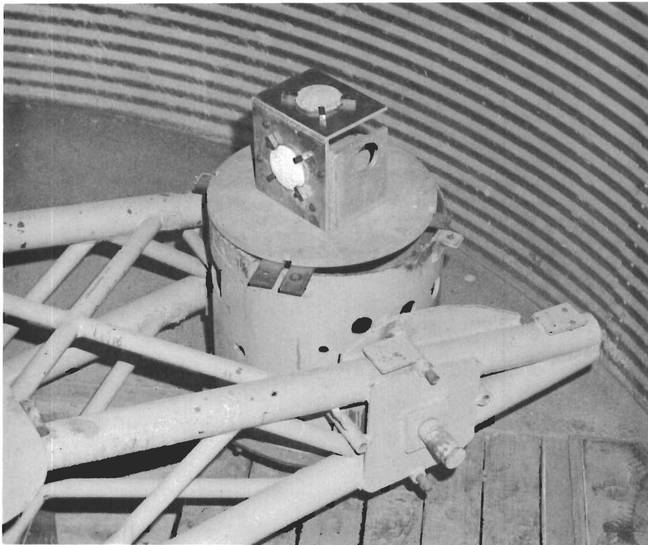
TEST UNIT MOUNTED IN JIG ON 60-INCH CENTRIFUGE ARM PRIOR TO TEST
