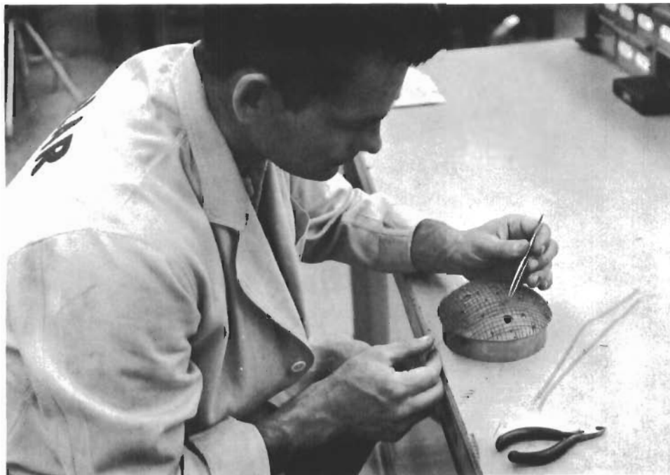
FIGURE 9. TUNGSTEN REINFORCEMENT COILS BEING APPLIED TO MESH FASTENED TO TUNGSTEN FORGING
