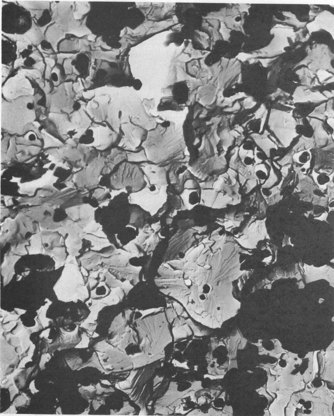
Fig. 60: Electron Micro-Fractograph of an Alloy 72,4% Fe, 12,6% Al, 4,5% Mo, 0,5% B, 10% TiC/Cr 3 C 2
