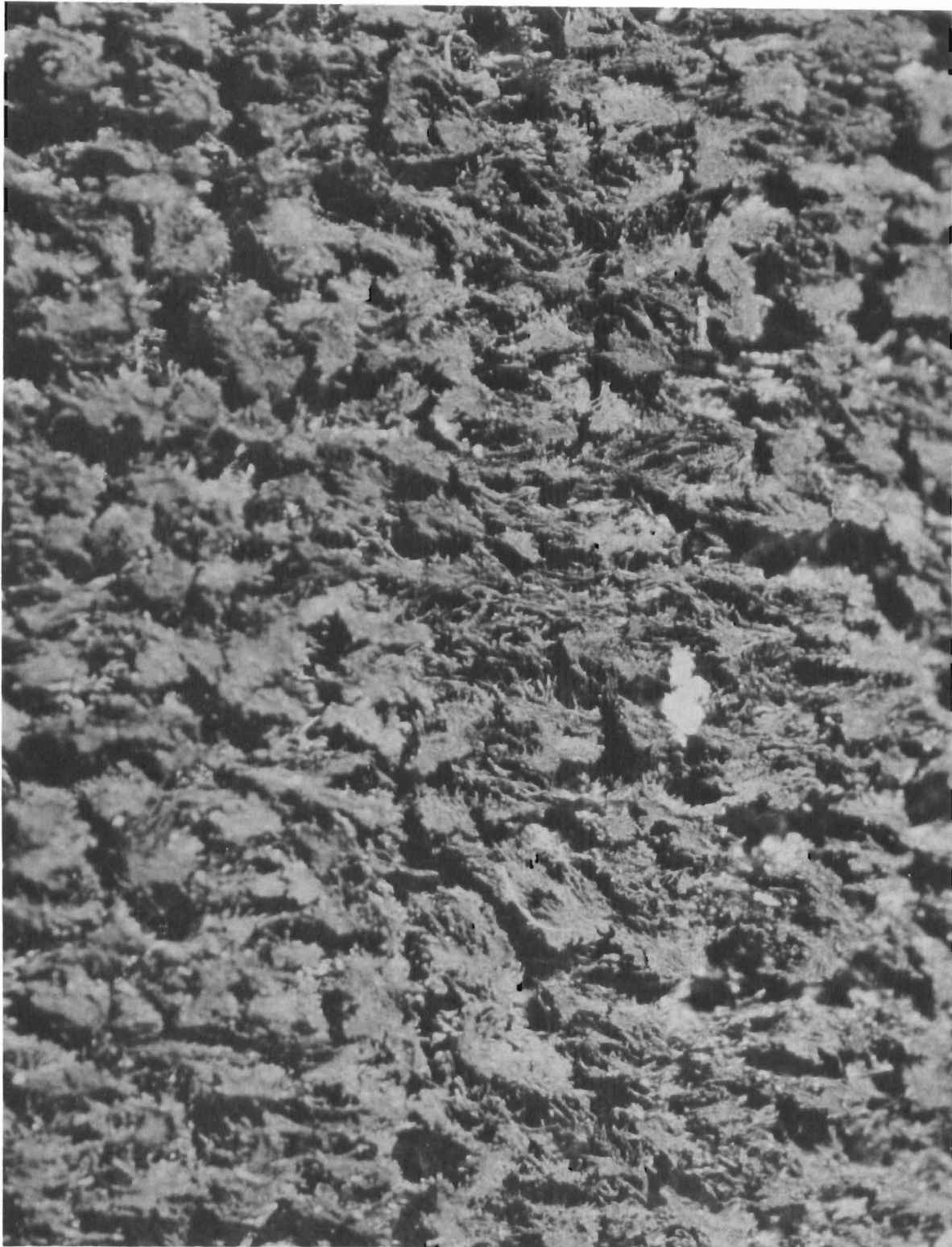
Figure 11. Carbonaceous Surface of Y-33 Specimen after Air Plasma Exposure (Enlarged 16 Optical Diameters)
