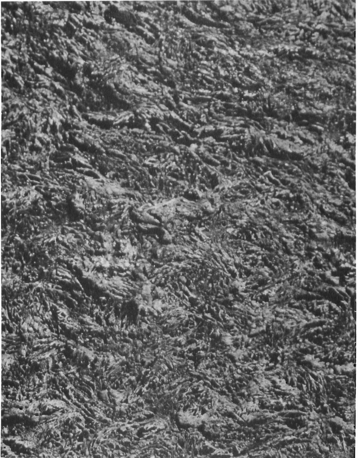
Figure 10. Carbonaceous Surface of Y-32 Specimen after Air Plasma Exposure (Enlarged 16 Optical Diameters)
