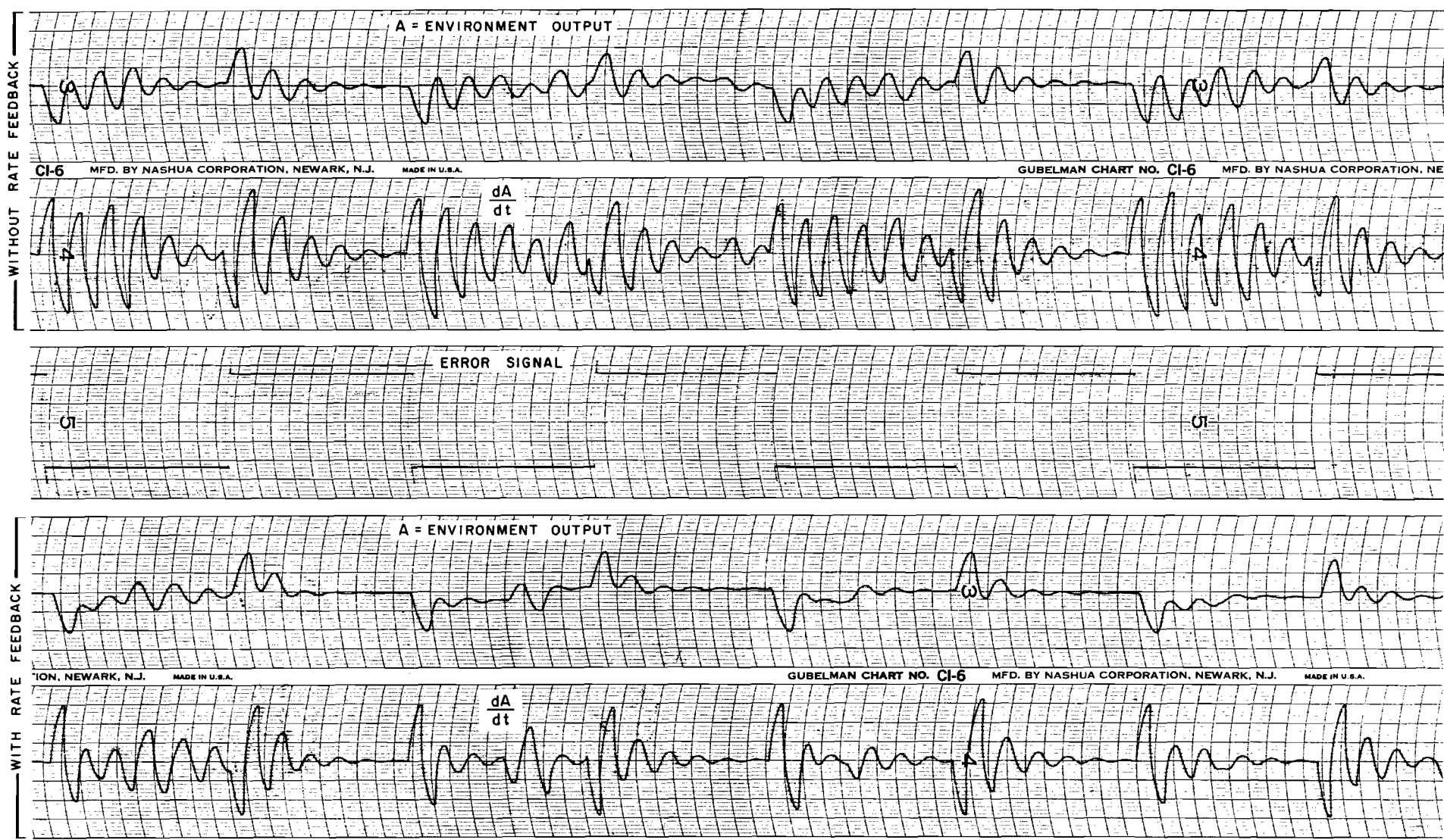
Figure 44. Analog Computer Test Run of Network Using Rate Feedback
