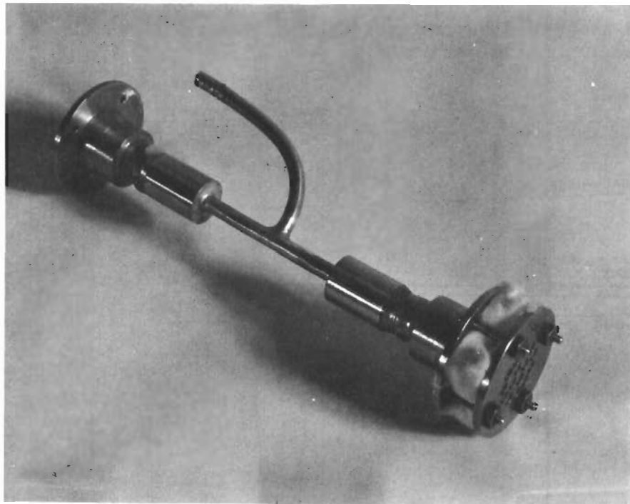
Figure 19. Two Capillary-Wick Feed System
