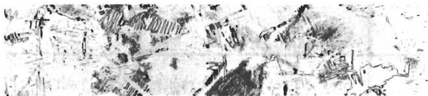
4d. Micro photograph of Fusion Zone Etchant: Modified Kroll's Etch, Magnification: 100X
