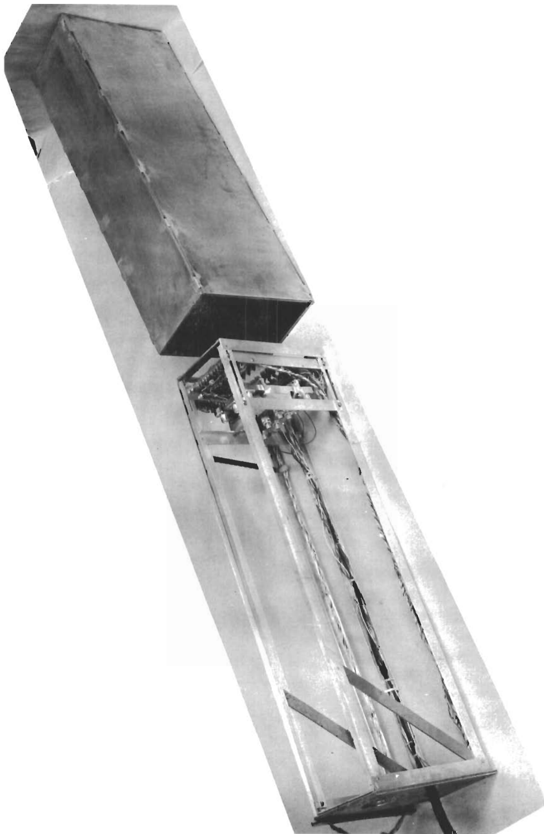
FIG. B-8 DIODE RACK ASSEMBLY WITH BORAL SHIELDING
