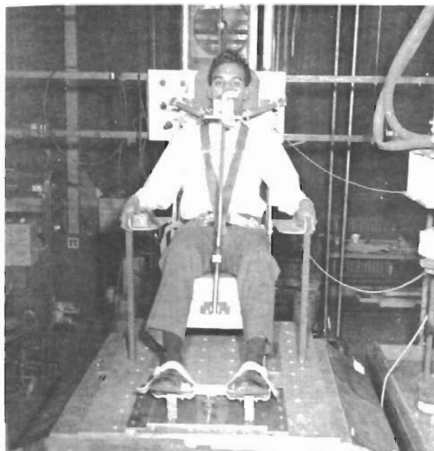
Figure 2. Illustrates Position of Subject and Restraint System (Front View)
