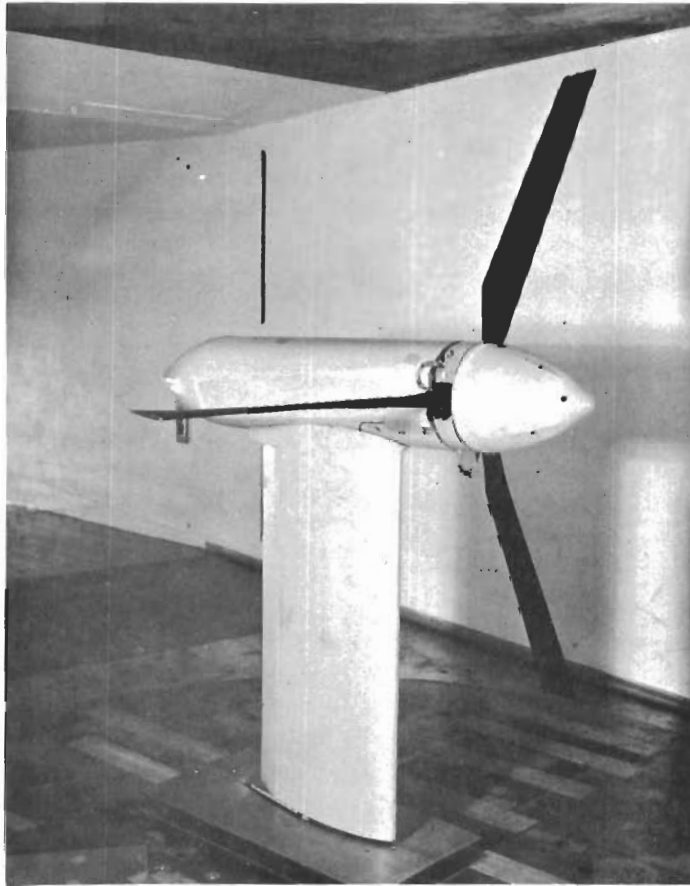
Figure 25. Model 213, 1/16-Scale Semispan Conversion Model Installed in Princeton University Low-Speed Wind Tunnel.
