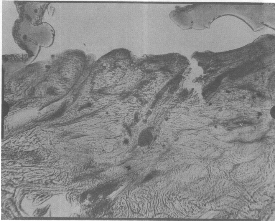
FIGURE 8. Sample 244 A-3. Break of the film and also beginning of erosion of the fibers.
