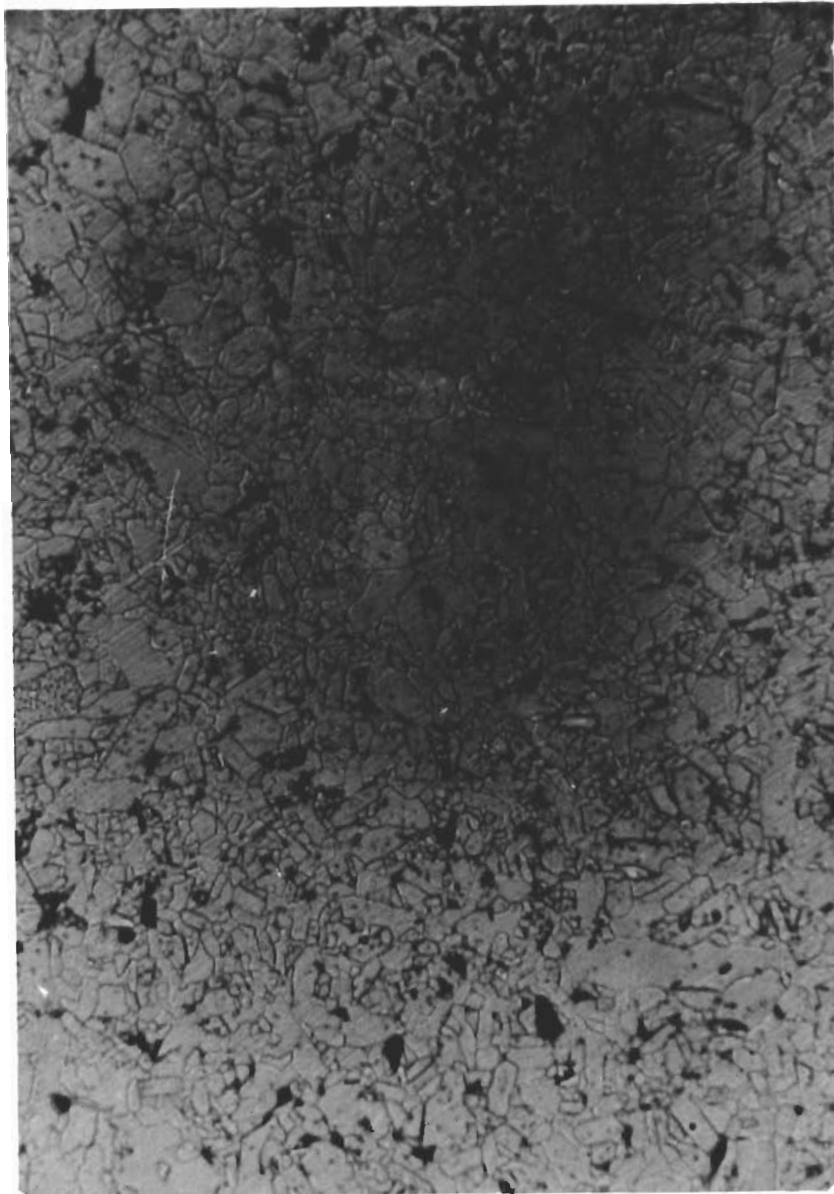
Fig. 8-19 Photomicrograph showing flash-etched surfaces of pressed and sintered high-purity \text{Al}_2\text{O}_3 doped prior to pressing with 100 ppm sodium oxide as \beta -alumina. (0.60 in. on the photomicrograph represents 100 microns on the actual surface.)
