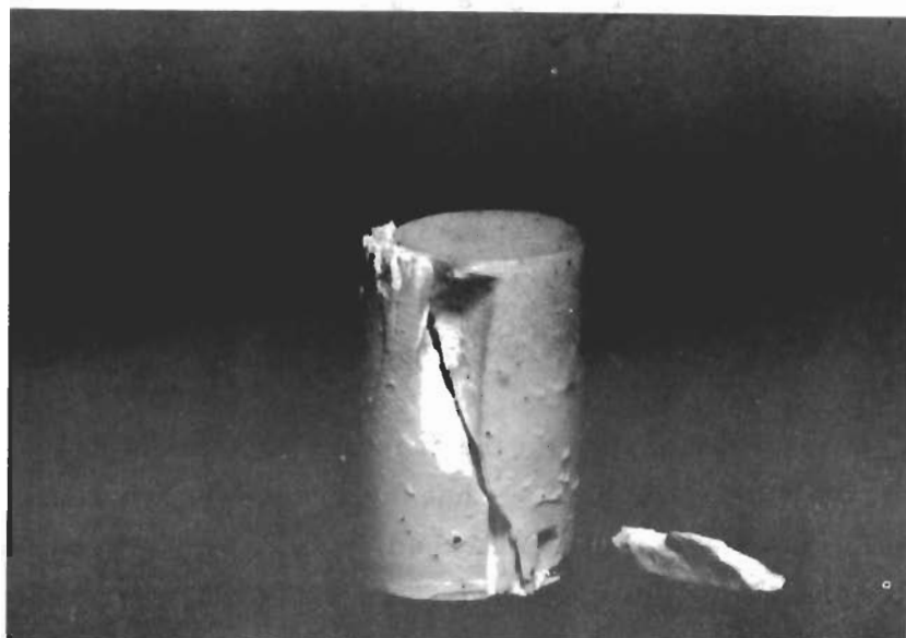
Fig. 4-7 POLYCRYSTALLINE MgO COMPRESSION SPECIMEN FRACTURED AT 1200°C
