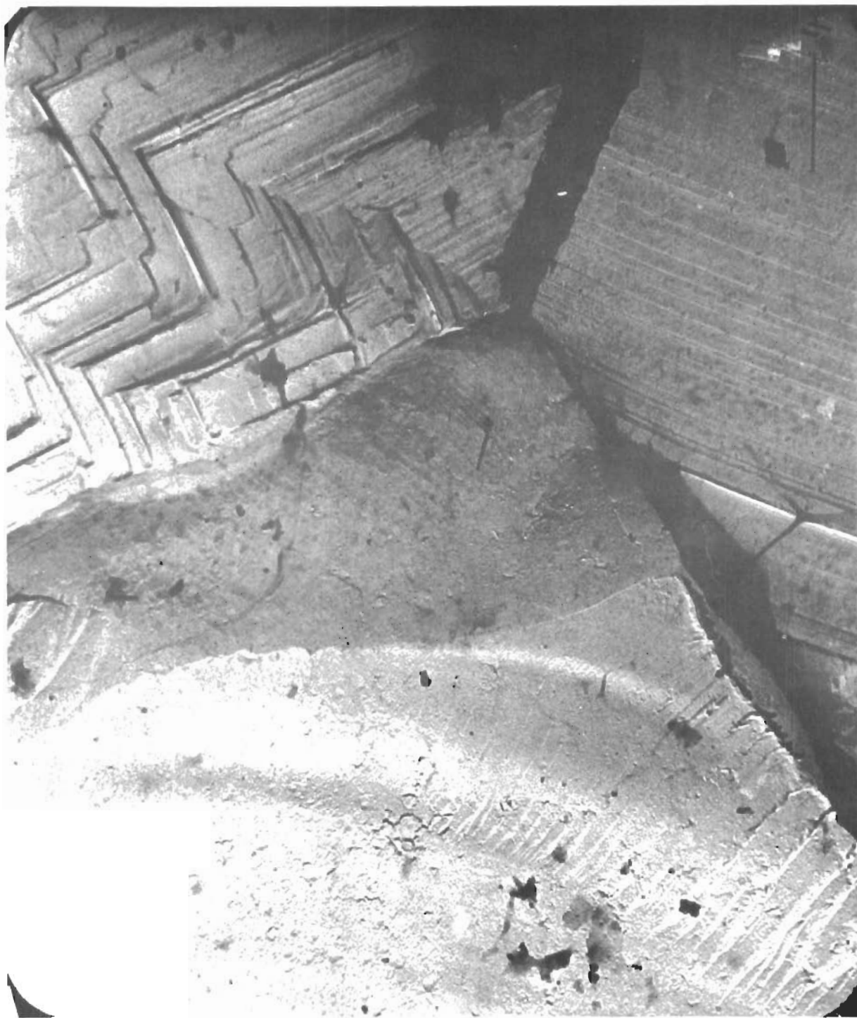
Fig. 6-17 EFFECT OF GRAIN ORIENTATION UPON FRACTURE SURFACE X24, 000
