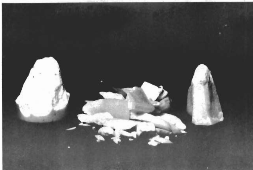
Fig. 4-7 POLYCRYSTALLINE MgO COMPRESSION SPECIMEN FRACTURED AT 1200°C
