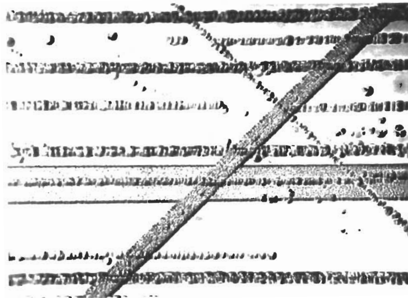
Fig. 10-13 THE REACTIVATION OF SHORT SLIP BAND SEGMENTS FOLLOWING AN ANNEAL (a) at 600°C, (b) at 800°C (X250)
