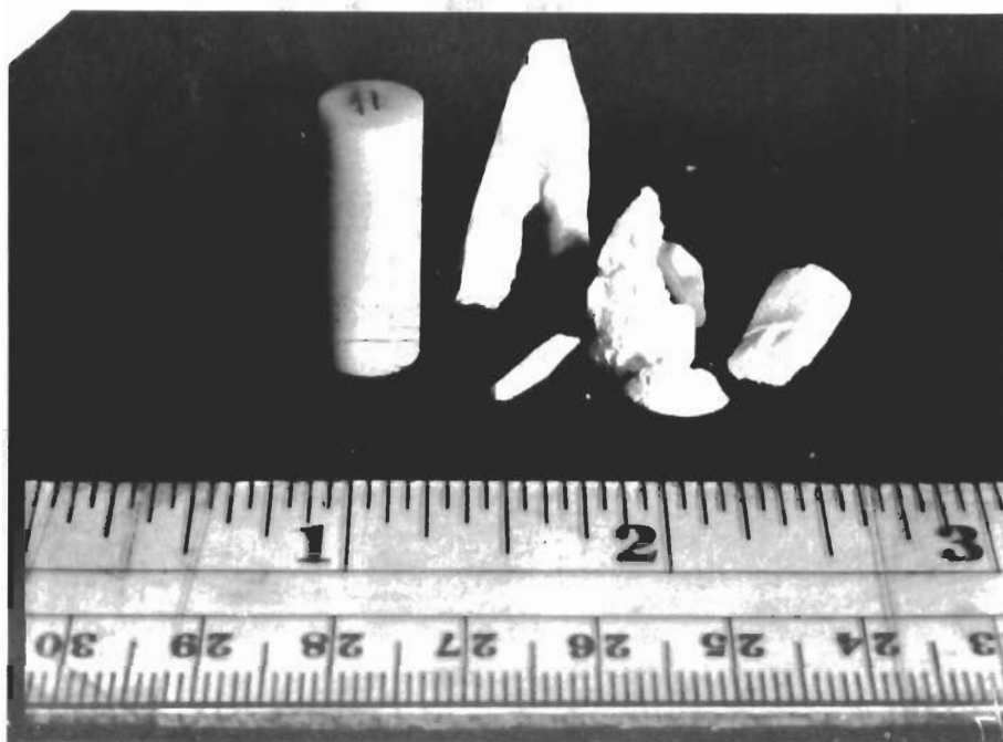
Fig. 4-14 LUCALOX SPECIMENS BEFORE AND AFTER TESTING UNDER COMPRESSIVE LOADING AT 1600°C Grain Size = 0.005 mm
