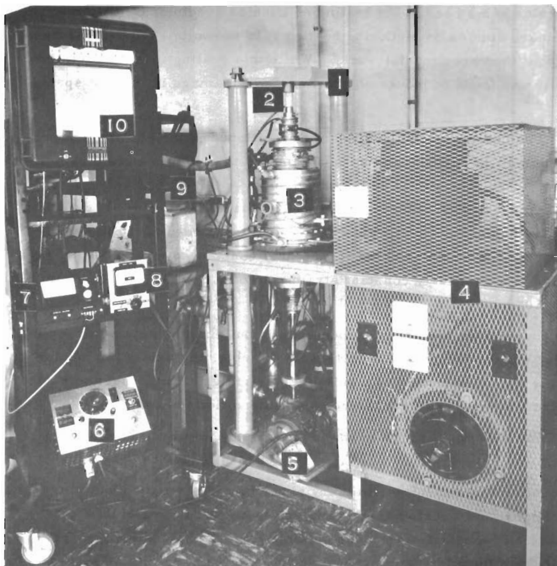
Fig. 4-2 FULL VIEW OF COMPRESSION TESTING UNIT
