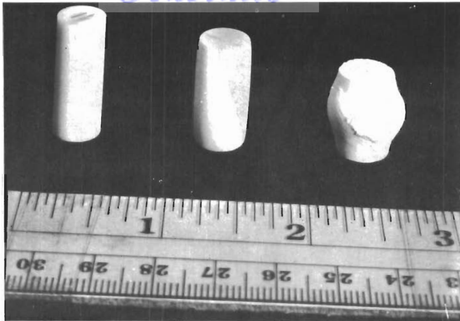
Fig. 4-16 LUCALOX SPECIMENS BEFORE AND AFTER TESTING UNDER COMPRESSIVE LOADING AT 1900°C Grain Size = 0.005
