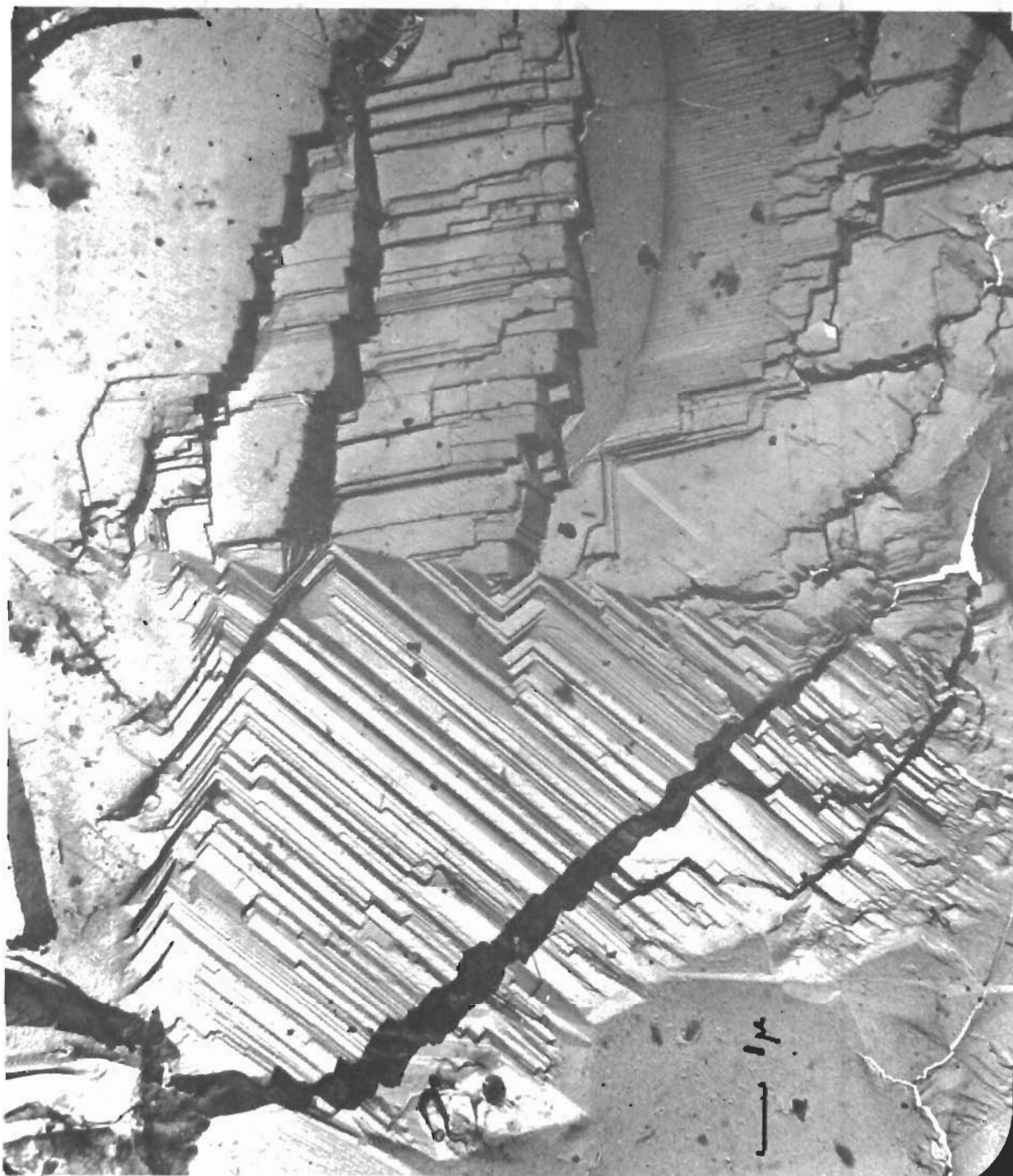
Fig. 6-18 FRACTURE SURFACE PATTERN ACROSS GRAIN BOUNDARY X12, 000
