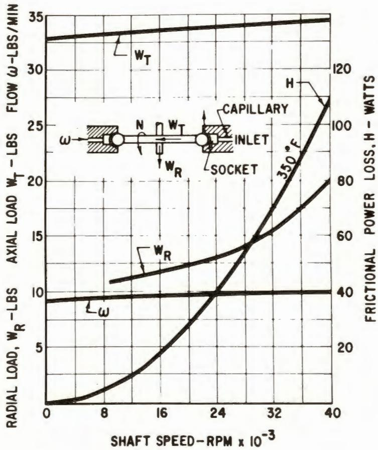
FIGURE 6. COMPOSITE 1/2-INCH DIAMETER HYDROSPHERE BEARING PERFORMANCE, LIQUID-MERCURY LUBRICATION
