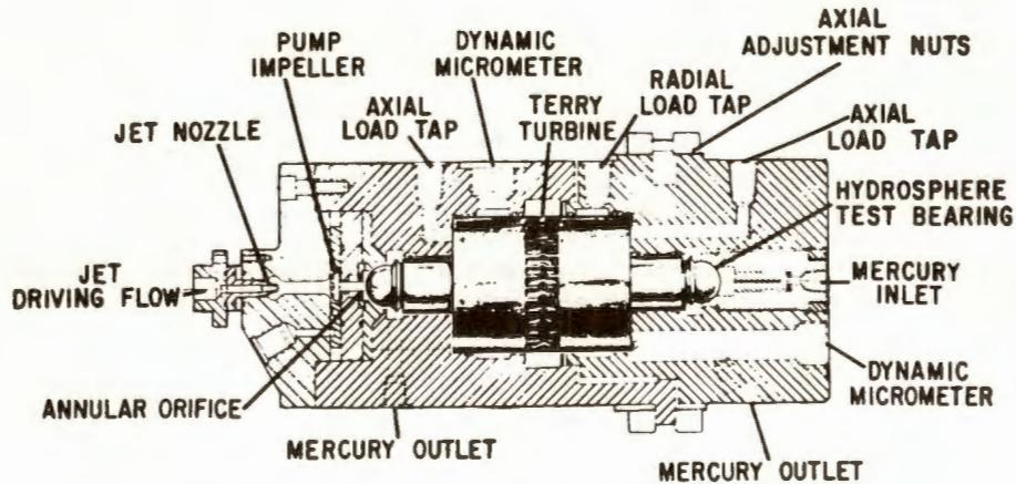
FIGURE 9. DUAL BEARING TEST FIXTURE
