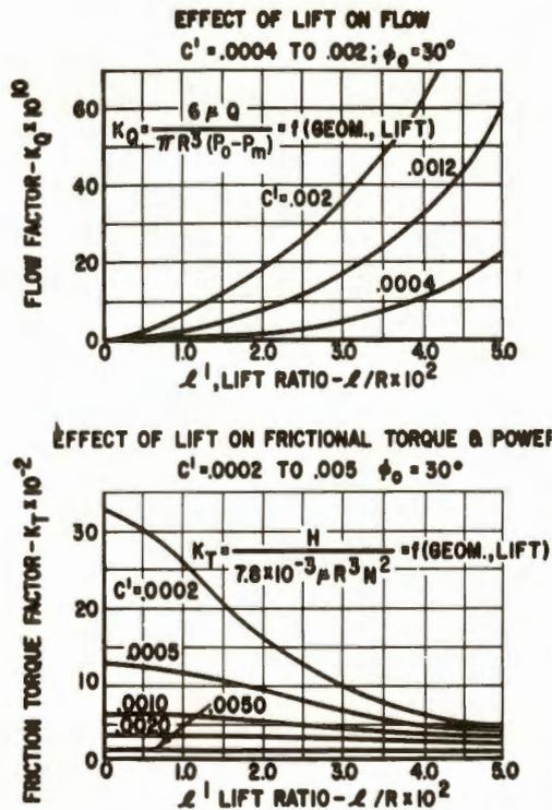
FIGURE 4. HYDROSPHERE BEARING, NON-DIMENSIONAL FLOW AND TORQUE FACTORS
