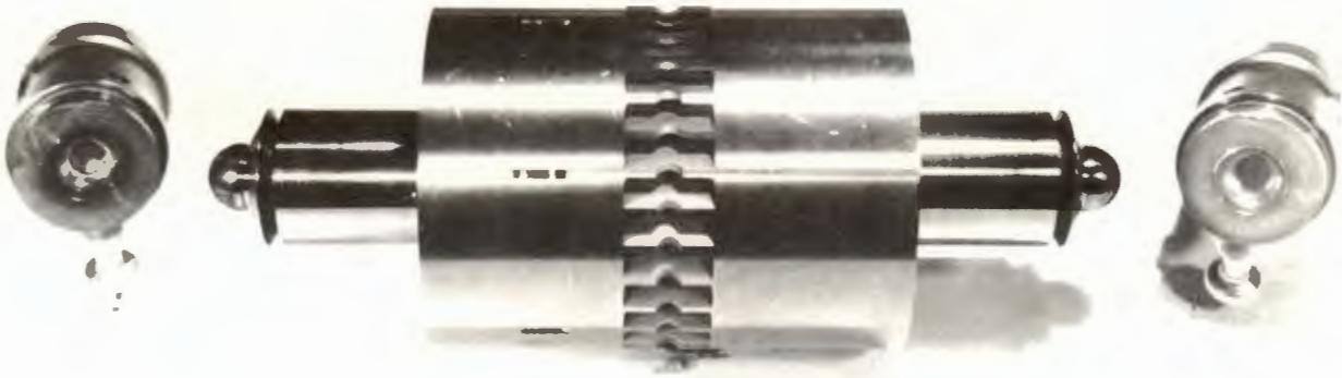
FIGURE 5. DUAL HYDROSPHERE BEARING SHAFT AND SOCKETS AFTER 104 HOURS OF LIQUID MERCURY OPERATION
