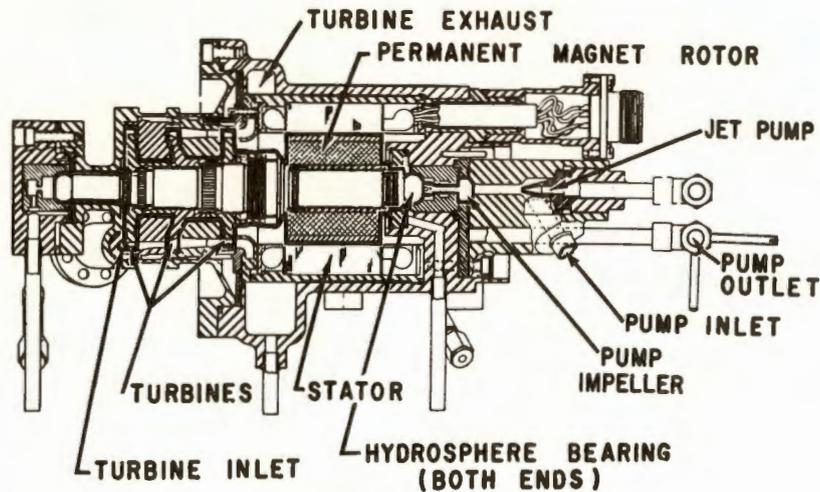
FIGURE 1. SNAP I TURBOMACHINERY PACKAGE
