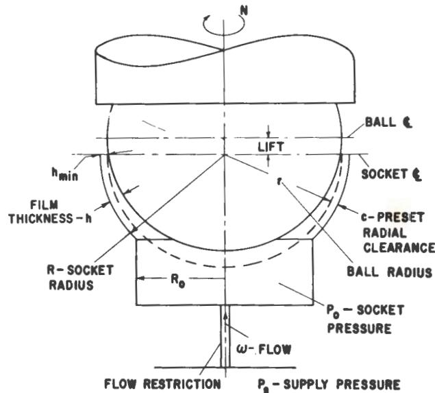
FIGURE 2. HYDROSPHERE BEARING ASSEMBLY
