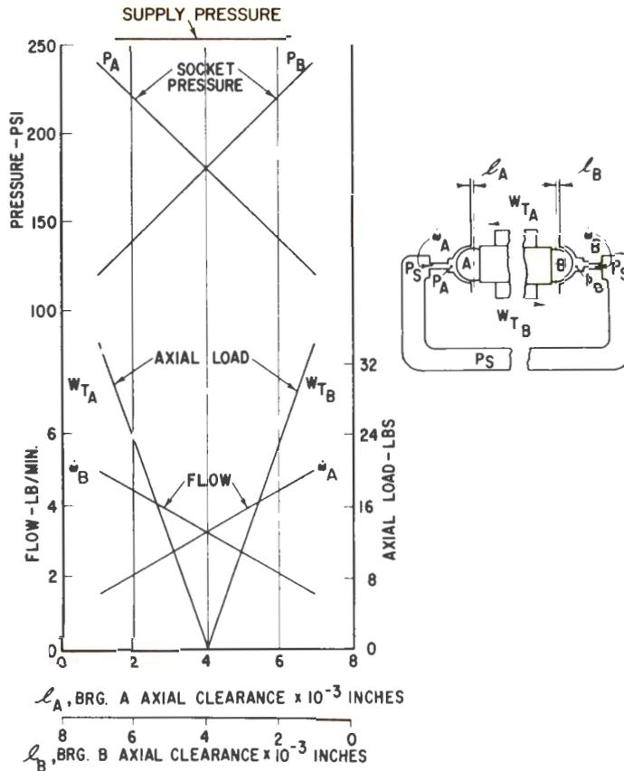
FIGURE 7. TYPICAL DUAL HYDROSPHERE BEARING CHARACTERISTICS
