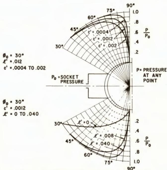
FIGURE 3. TYPICAL HYDROSPHERE BEARING FILM PRESSURE DISTRIBUTION
