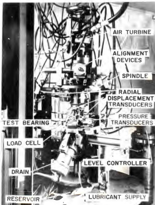
FIGURE 8. SINGLE HYDROSPHERE BEARING TEST RIG
