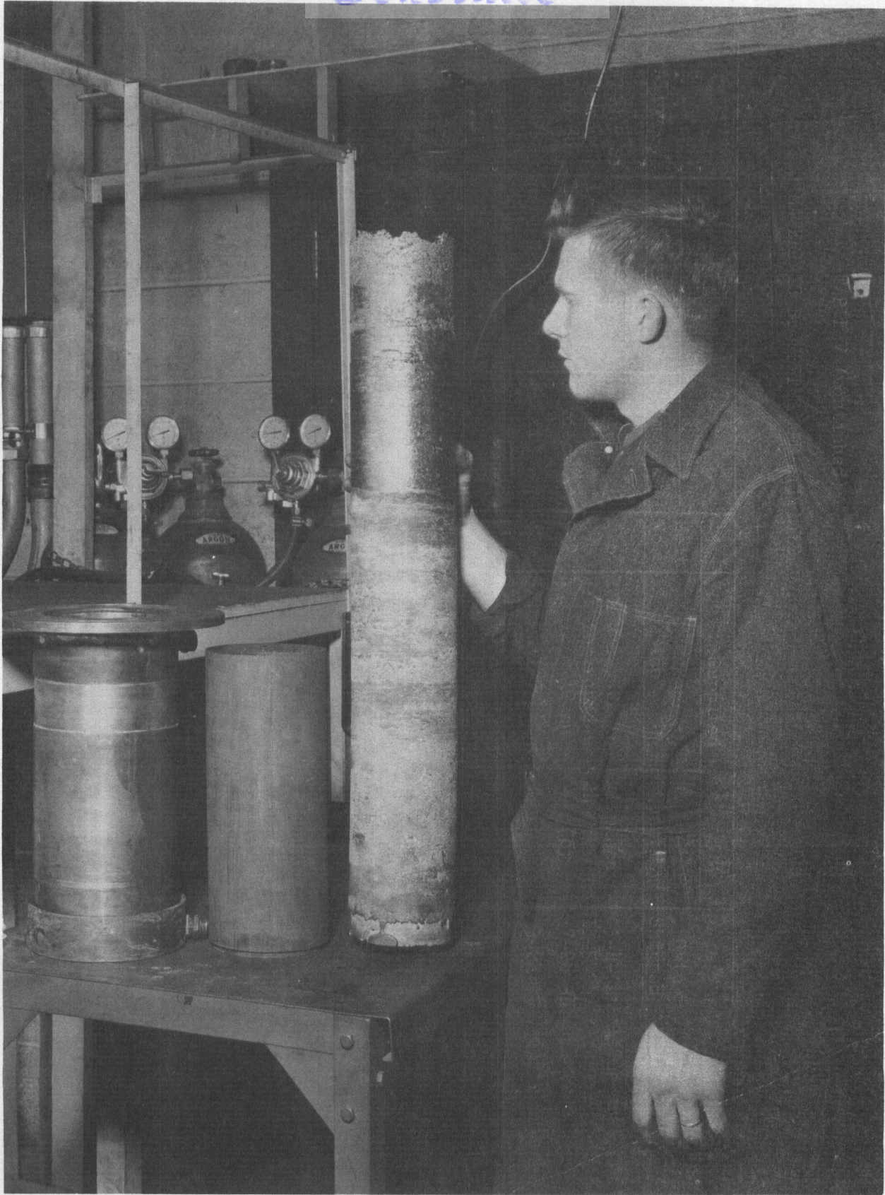
FIG. 4 - SIX INCH CRUCIBLE WITH GRAPHITE LINER AND A 113-POUND Ti-6% Al INGOT AS CAST
