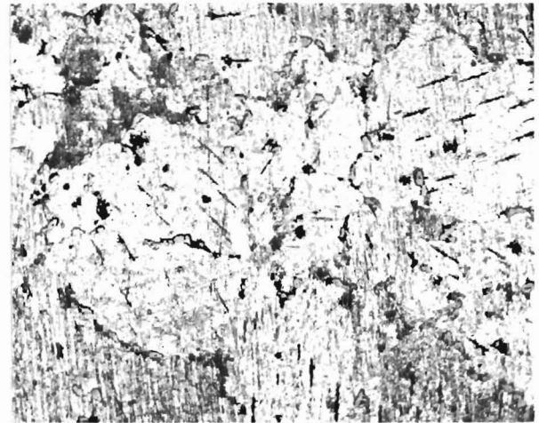
Figure 29. Erbium, heat treated at 1000°C, slow cooled. Nitric acid etch. 250X.
