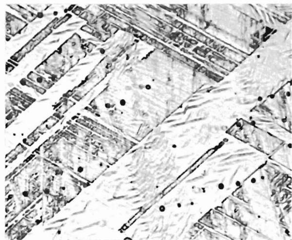
Figure 90. Cobalt- \frac{1}{4} % erbium, as arc-melted. Electro-polished. 500X.
