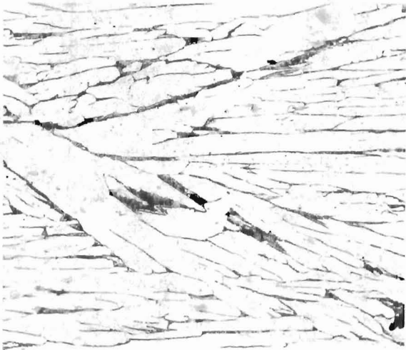
Figure 100. Cobalt-25% erbium, as arc-melted. Compound plus eutectic. Cobalt #1 etch (60 ml hydrochloric, 15 ml nitric, and 15 ml acetic acids with 15 ml distilled water). 100X.
