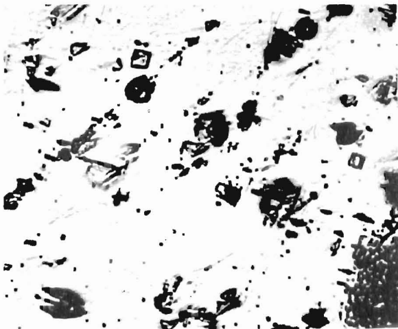
Figure 7. Beryllium - 1% erbium, as arc-melted. Cubic crystals are \text{Be}_{13}\text{Er} . Microporosity appears as black circles. 5% HF in methanol etch. 500X.
