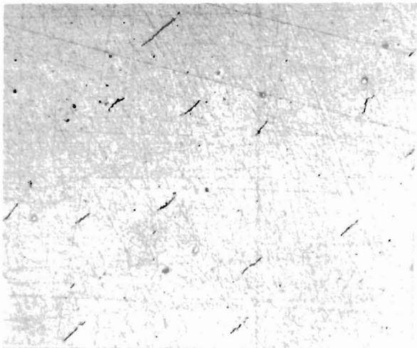
3479 Figure 69. Distilled yttrium, oxygen content 0.04%. Entire area within one grain. Oxide platelets plus small crystal- lites. Unetched. 250X.
