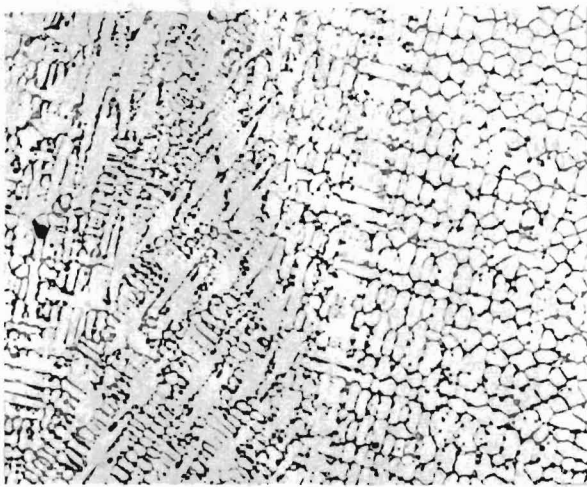
Figure 108. Nickel-1% yttrium, as arc-melted. Dendritic primary nickel plus eutectic. Electro-polished, Carapella's etch. 100X.
