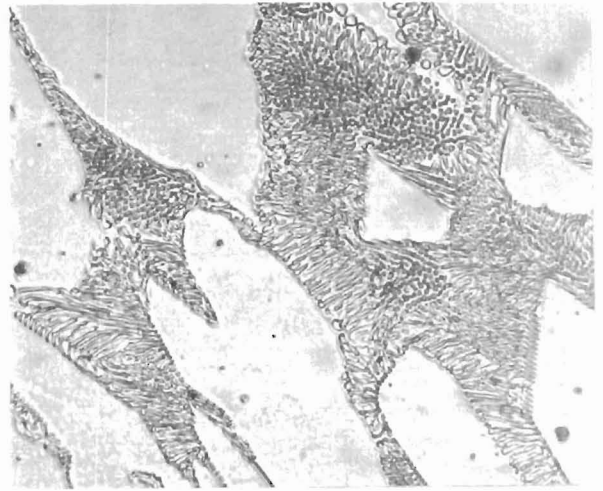
Figure 101. Cobalt-25% erbium, as arc-melted. Detail of eutectic rich region. Electro-polished. 750X.
