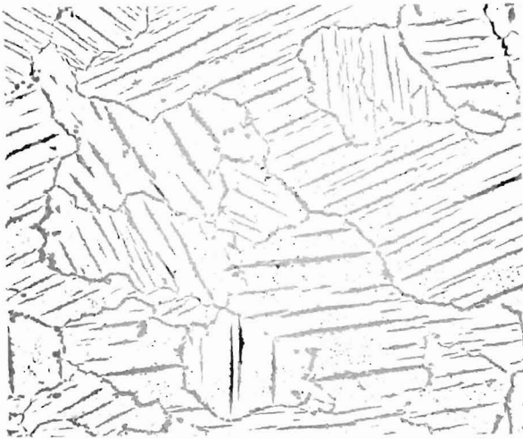
Figure 45. Erbiun-10% \text{Er}_2\text{O}_3 , as arc-melted. Oxide principally in grain boundaries and as platelets within grains. Unetched. 100X.
