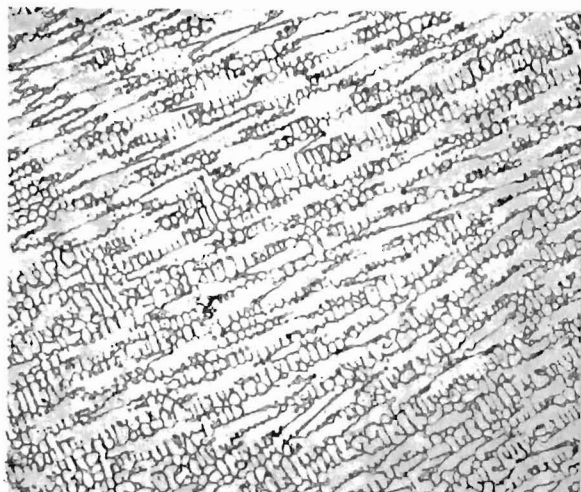
Figure 95. Cobalt-5% erbium, as arc-melted. Primary dendritic cobalt with eutectic. Electro-polished. 100X.
