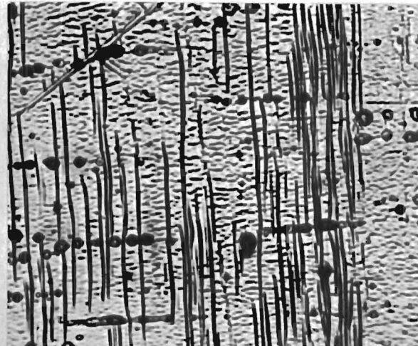
Figure 92. Cobalt- \frac{1}{2} % erbium, as arc-melted. Detail of eutectic and banded structure. Electro-polished. 500X.
