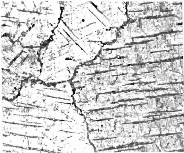
Figure 26. Yttrium - 50% erbium, heat treated at 1000°C, slow cooled. Nitric acid etch. 250X.
