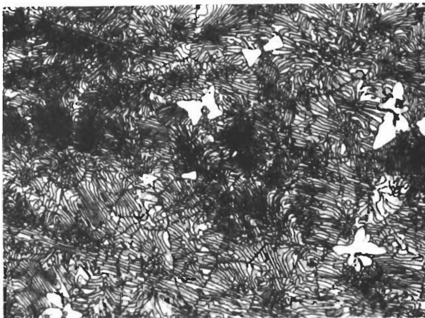
Figure 23. Ti-V-C (5-81-14 At.%), Melted and Rapidly Cooled. X600 Eutectic Solidification Structure at the Three-Phase Boundary \beta + \gamma + \delta , with Traces of Binary Metal Phase.
