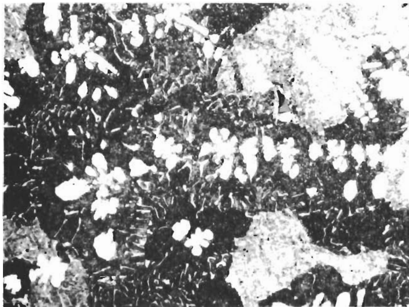
Figure 20. Ti-V-C (20-70-10 At.%), Melted and Quenched. X600
