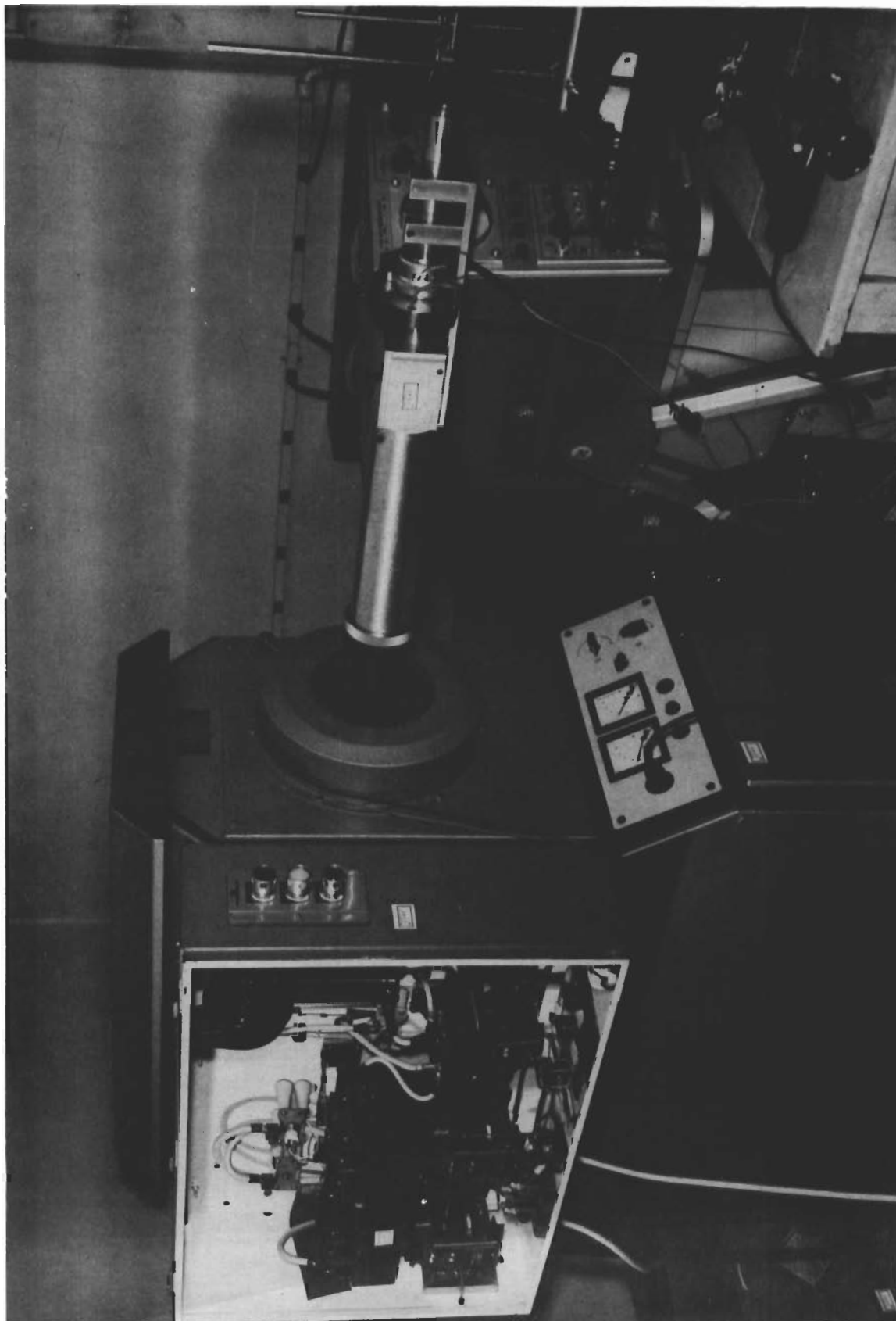
Figure 4. ZEISS LIGHT COAGULATOR MODIFIED FOR PULSING
