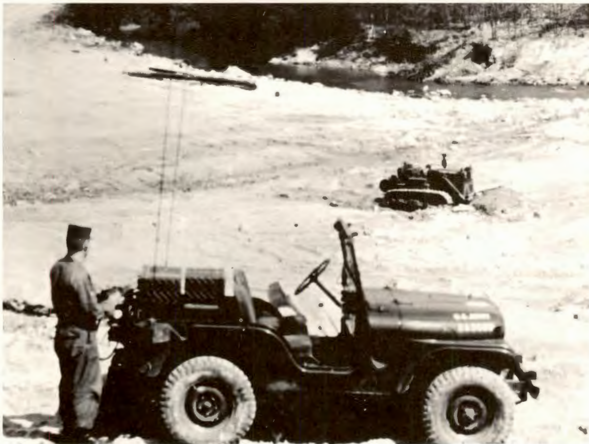
Figure 16. A Remotely Controlled Bulldozer
