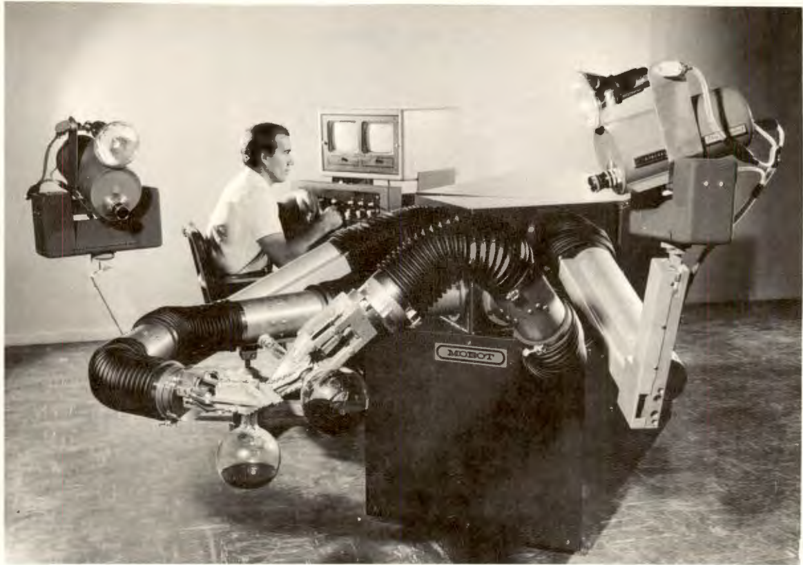
Figure 1. A Typical Electronically Commanded, Remote-Handling System
