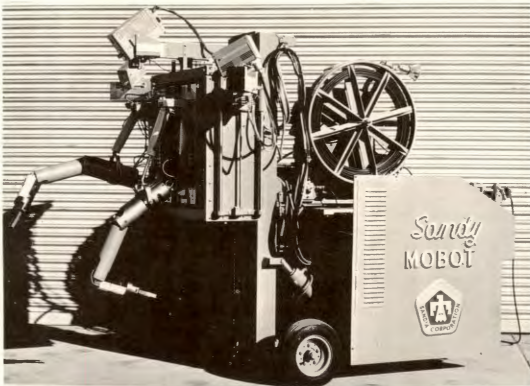
Figure 11. The Mobot Mark I Heavy-Duty, Remote-Handling System
