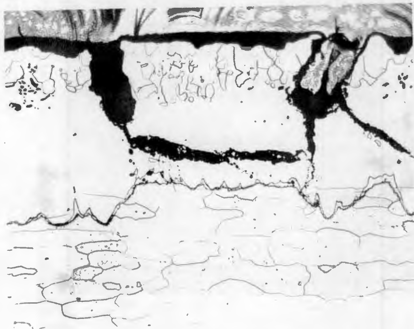
Figure 16. After 22 hours at 2700°F. Mag. 250 X
