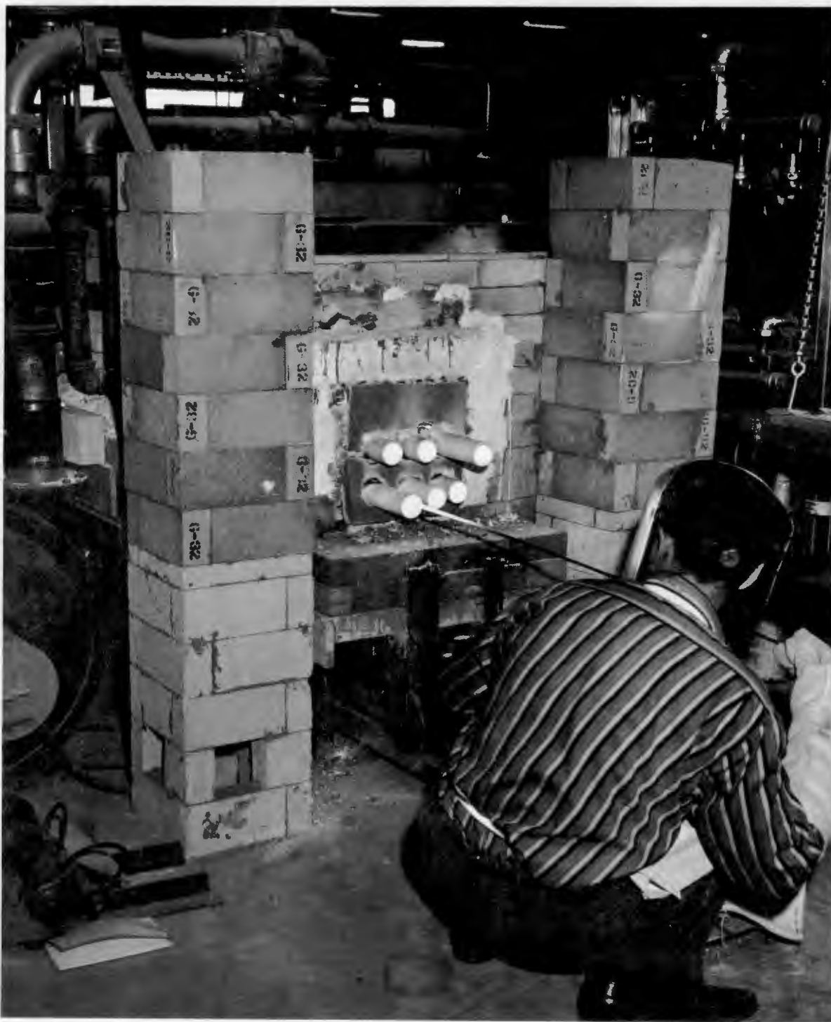
Figure 4. Tube Furnace Used for Oxidation Testing Specimens at 2700°F.
