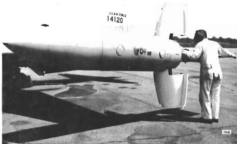
FIGURE 1 DRAG PETALS, WITHOUT PETAL EXTENSIONS, ON T-33 TIP TANKS
